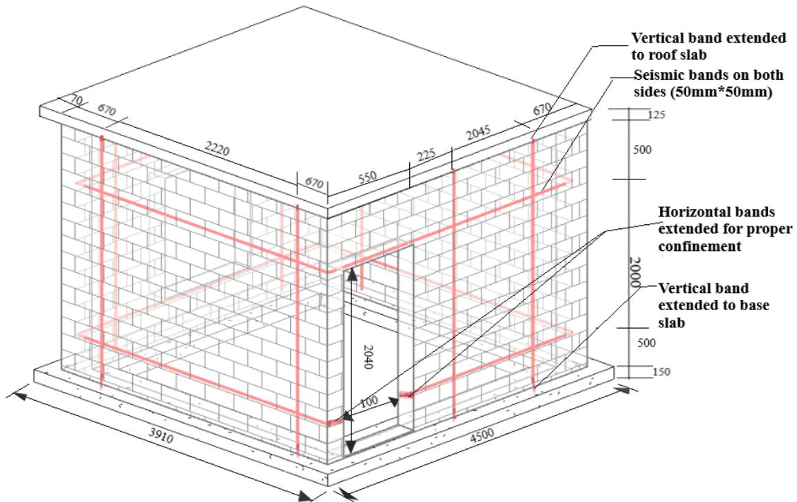
Fig. 4 – Schematic diagram of S\_URBM specimen with horizontal and vertical seismic bands at strategic locations (All dimensions in mm)
