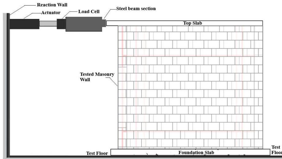
Fig.6 – Schematic diagram showing loading system
