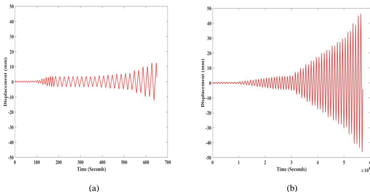
Fig.8 – Recorded loading history for: (a) URBM and (b) S\_URBM specimens (as per FEMA 461)
