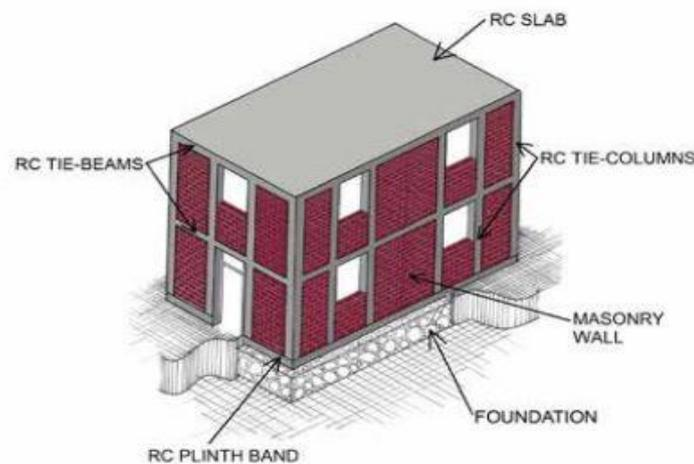
Fig. 1 – Components of confined masonry[4]
