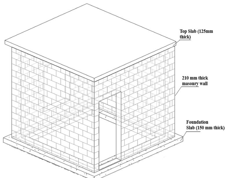
Fig. 2 – Schematic diagrams showing URBM specimens constructed on strong test floor
