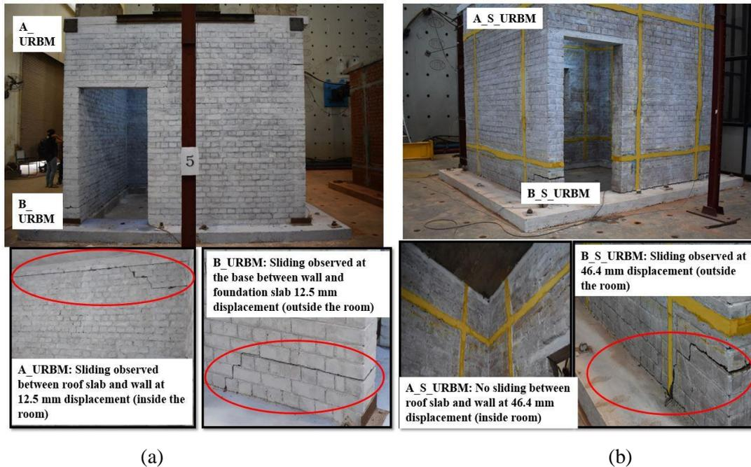
Fig.10 – Crack pattern observed at the end of the test for: a) URBM and b) S\_URBM specimens
