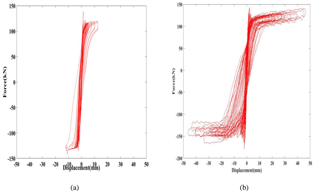
Fig.9 – Force-roof displacement behaviour obtained from slow cyclic tests on: a) URBM specimen, and b) S\_URBM specimen
