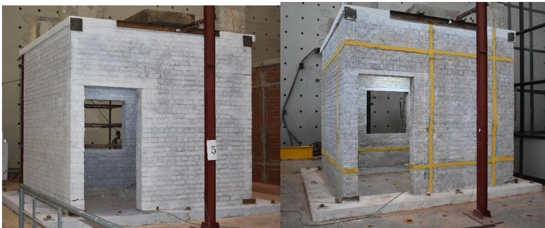
Fig.5 – Full-scale masonry structures : a) Unreinforced Brick Masonry (URBM), and b) Strengthened/Retrofitted Brick Masonry (S\_URBM)
