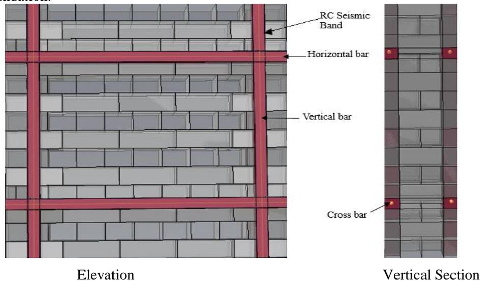
Fig. 3 – Schematic diagram showing the main components of semi-confined masonry wall
