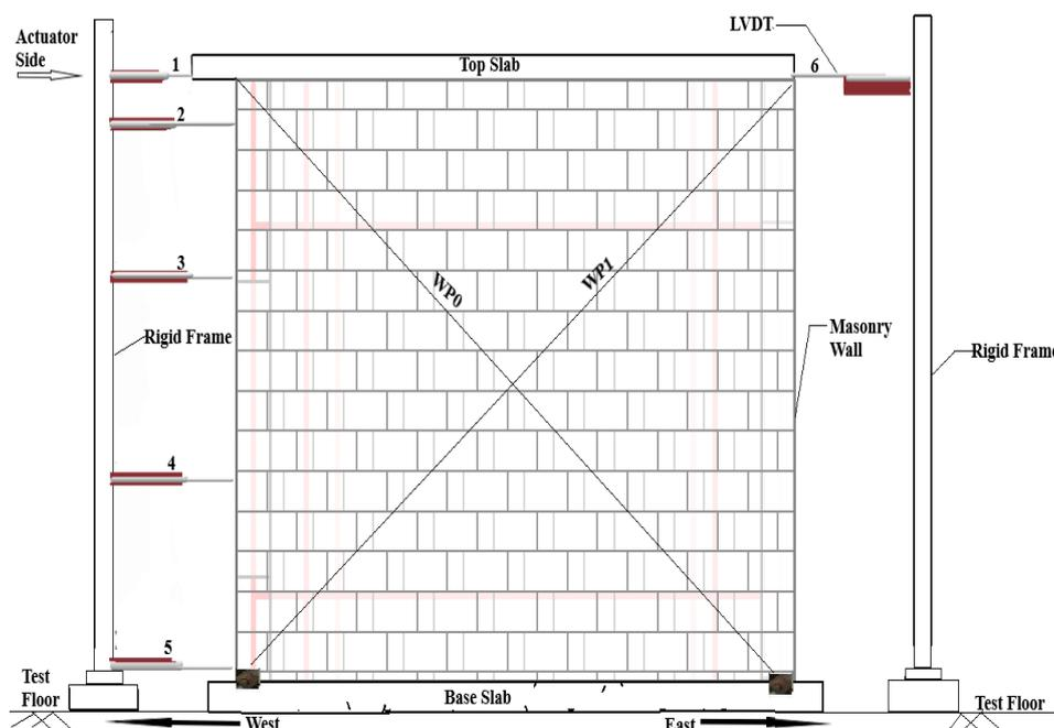
Fig.7 – Positions of LVDTs and wire Potentiometers in URBM and S\_URBM structures (Right face of wall from actuator side. Similar configuration was adopted for left face too.)
