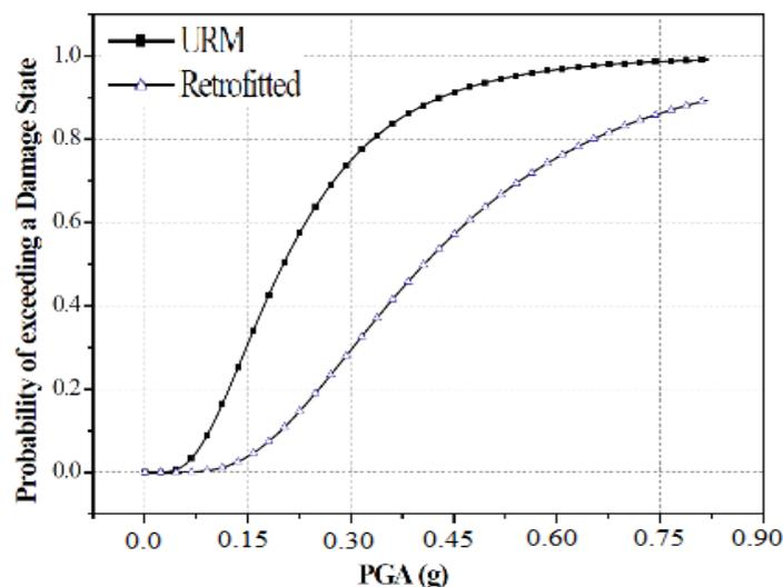
Fig.11 – Fragility Curves for URBM (URM) and S\_URBM (Retrofitted) structures
