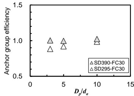
Figure 7. The Anchor group efficiency -  $D_p/d_a$  relationship due to difference in anchor strength
