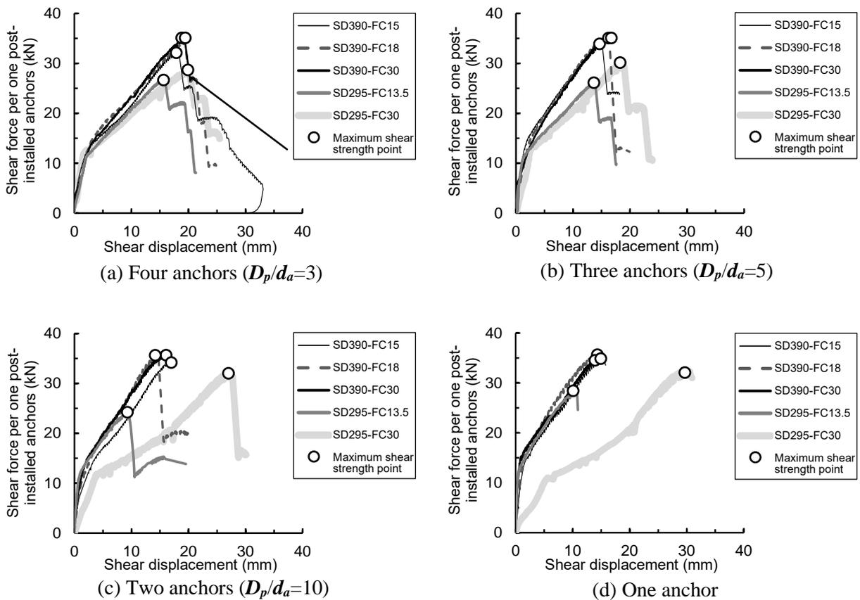
Figure 4. The shear force – shear displacement relationships
