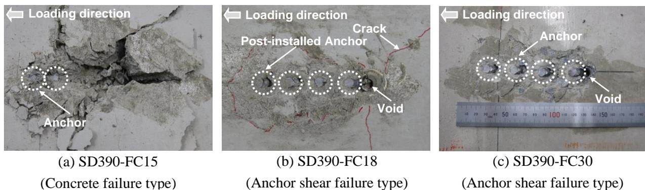
Figure 3. Major damage patterns of specimens
