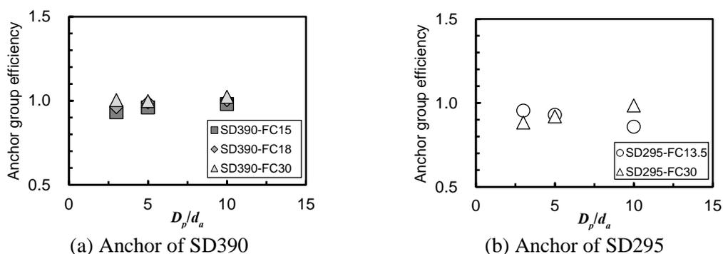
Figure 6. The Anchor group efficiency -  $D_p/d_a$  relationships
