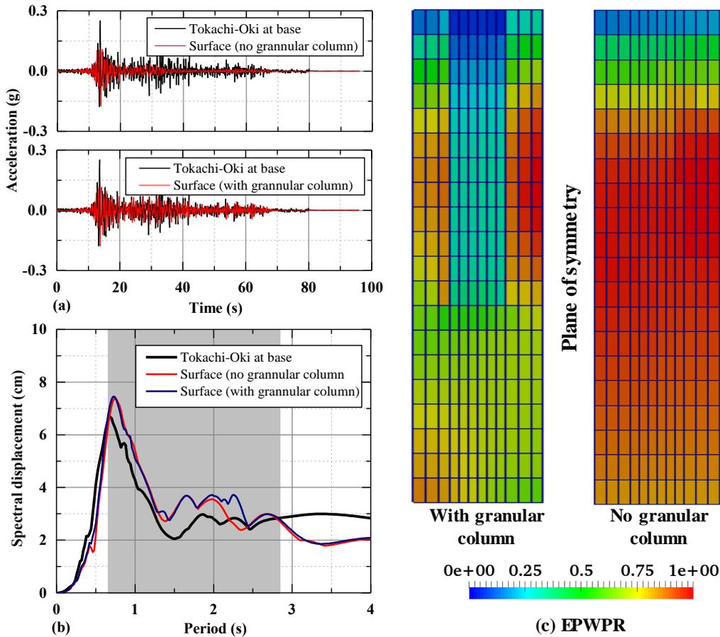
Fig. 7 Deterministic analysis ( $D_R = 50\%$ ): (a) accelerations at surface ( $Z = 0$  m) in comparison with applied Tokachi-Oki ground motion at base, (b) displacement response spectra (with 5 % damping), and (c) distribution of EPWPR on XZ plane ( $Y=0$ ) at Time,  $t = 18$  s
