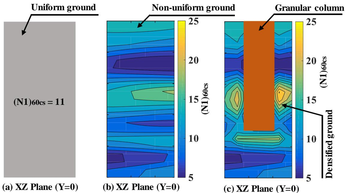
Fig. 5 A typical scenario of the ground condition at XZ Plane ( $Y=0$ ; see Fig. 2): (a) uniform ground, (b) non-uniform ground, and (c) non-uniform ground densified during to installation of granular column
