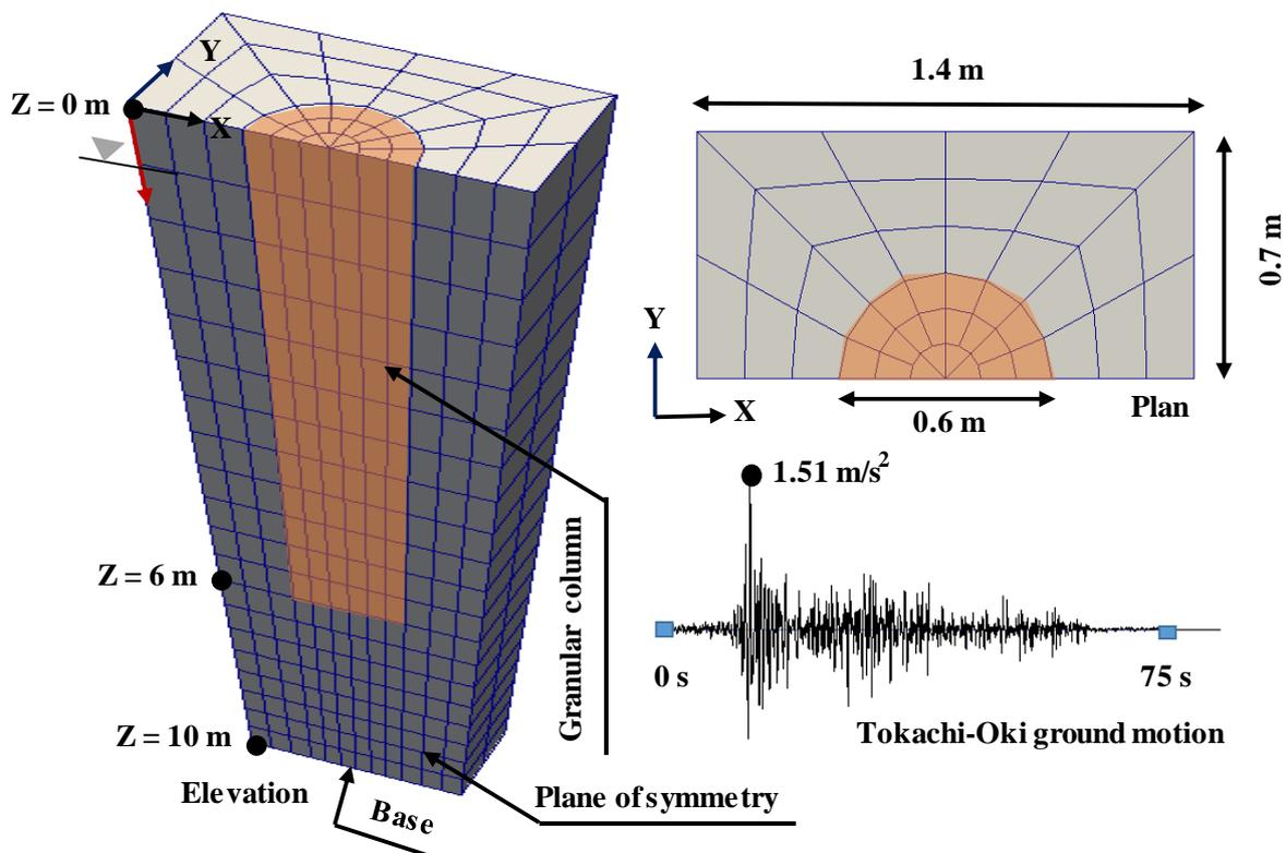
Fig. 2 Three-dimensional (3D) numerical model
