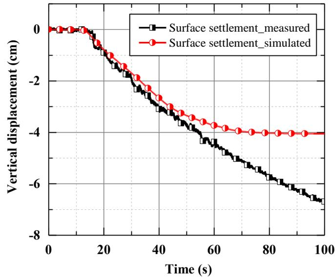
Fig. 4 The Response of the calibrated PDMY02 Model at the system level
