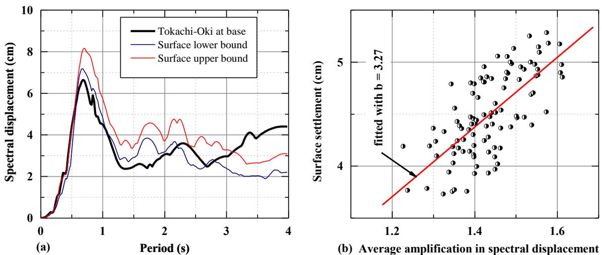
Fig. 8 Stochastic analyses: (a) upper and lower bound of displacement response spectra (with 5 % damping) at the surface ( $Z = 0$  m) and (b) correlation between average surface settlement and average amplification (period  $T = 0.5 - 3.0$  s) of spectral displacement
