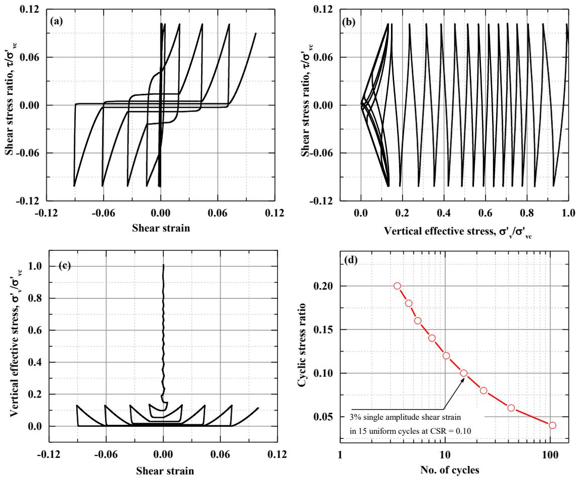
Fig. 3 The response of the calibrated PDMY02 Model at the element level
