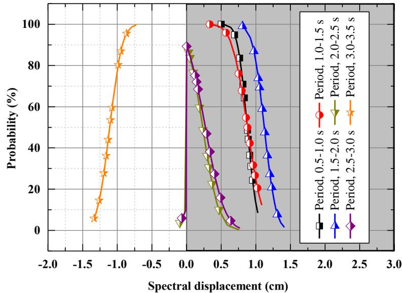
Fig. 9 Probability of deviation of average spectral displacement (for different period range) from their respective deterministic values
