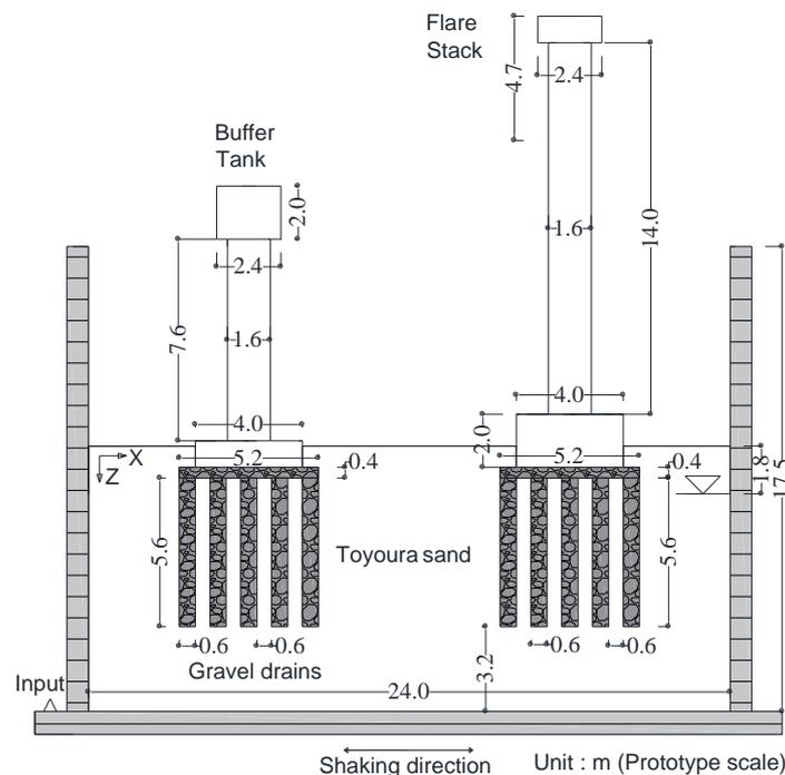
Fig 1. Centrifuge model configuration in the prototype scale
