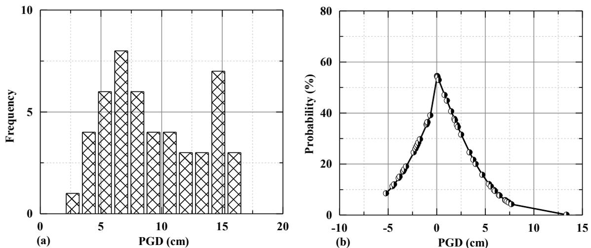
Fig. 10 Peak ground displacement: (a) stochastic distribution and (b) probability of deviation of PGD from the deterministic value of 8.15 cm
