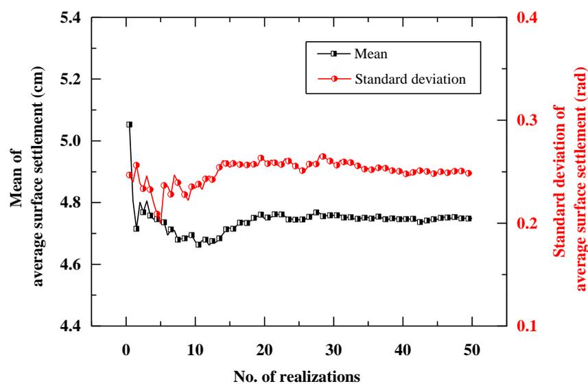
Fig. 6 Convergence check for sufficiency of the number of realizations
