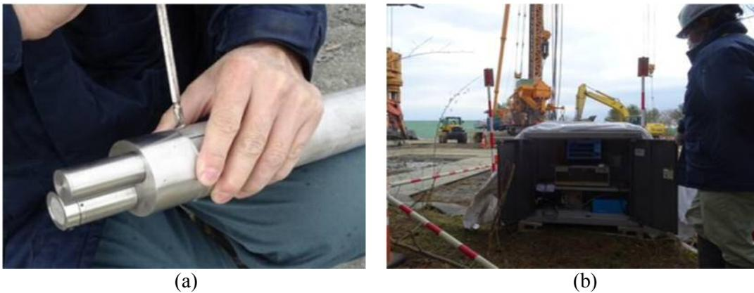
Fig. 3 – Photos showing: (a) accelerometer and pore pressure gauge used in the test; and (b) condition during the test.
