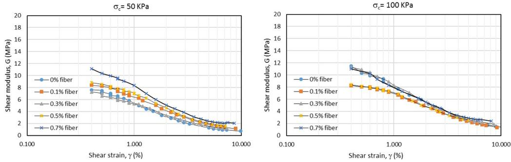
Fig. 6 Shear modulus vs. shear strain curves at confinement pressures of 50 KPa (left) and 100 KPa (right)
