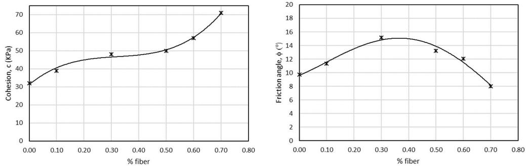
Fig. 4 Left: change in soil cohesion with fiber content; right: change in the soil internal friction angle with fiber content
