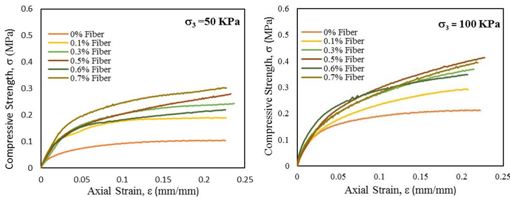
Fig. 1 Stress vs. strain for confinement pressures of 50 KPa (left) and 100 KPa (right)
