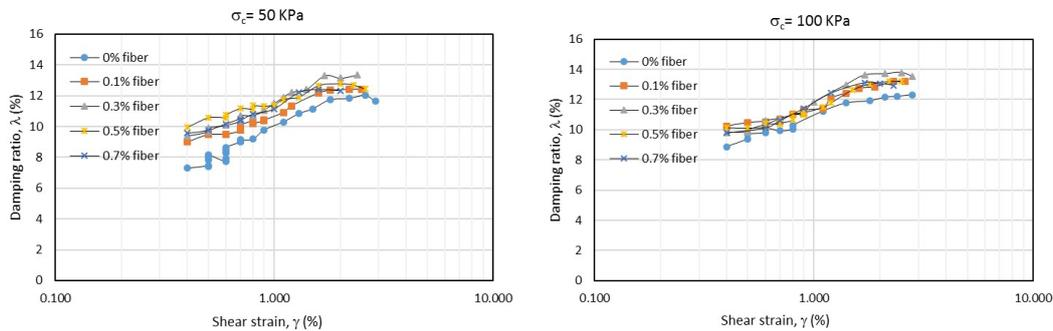
Fig. 8 Damping ratio vs shear strain for confinement pressures of 50 KPa (left) and 100 KPa (right)
