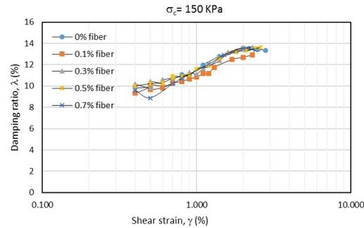
Fig. 9 Damping ratio vs shear strain for a confinement pressure of 150 KPa
