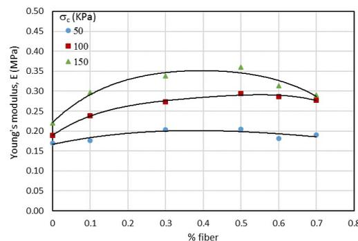
Fig. 5 Young's modulus for soil samples with different fiber percentages and confinement pressures
