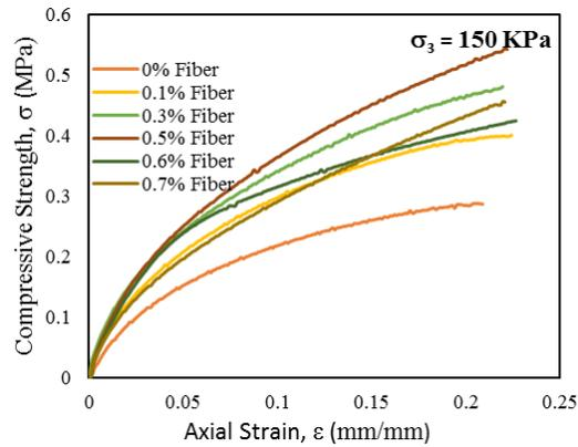
Fig. 2 Stress vs. strain for a confinement pressure of 150 KPa
