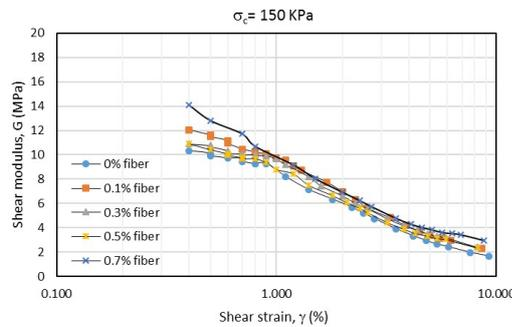
Fig. 7 Shear modulus vs shear strain for a confinement pressure of 150 KPa
