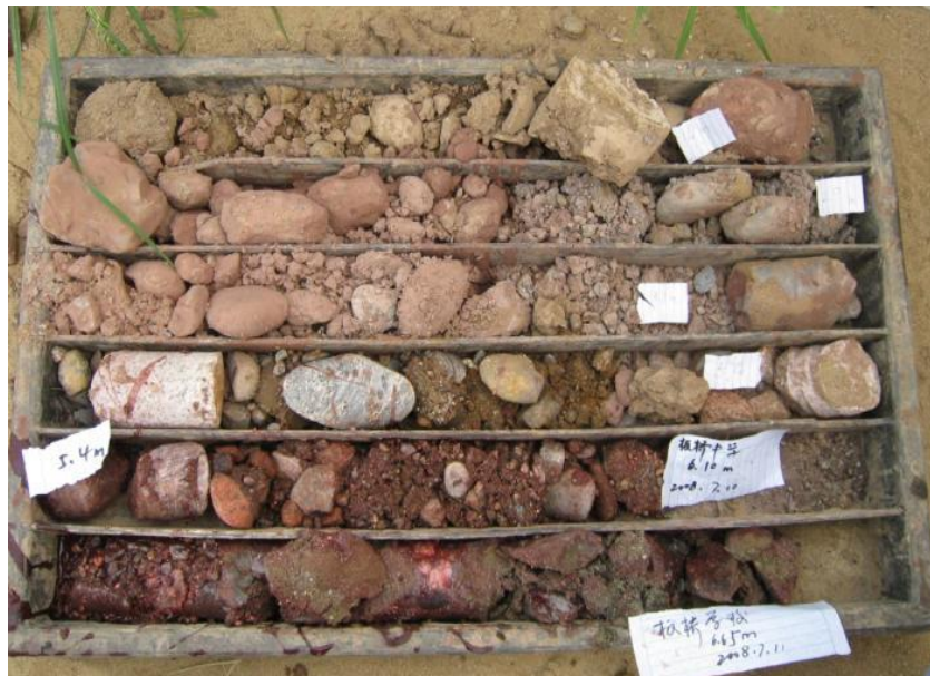
Figure 2. Typical extracted core samples
