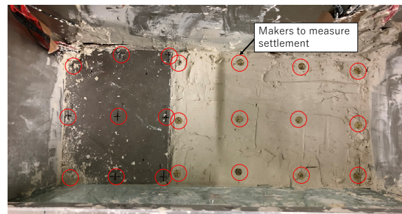
Fig. 7. Top view of single clay layer before the initial flight. Left grey part is the steel plate to give equivalent load to an embankment.
