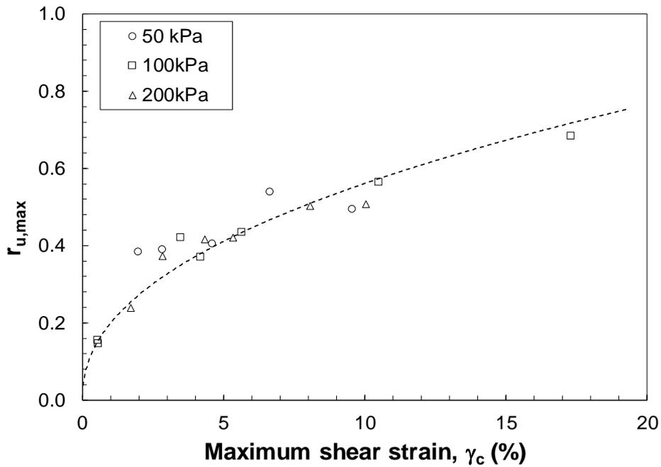
Fig. 3 - Generation of maximum excess pore pressure ( $r_{u,max}$ ) in Toronto peat as a function of  $\gamma_c$
