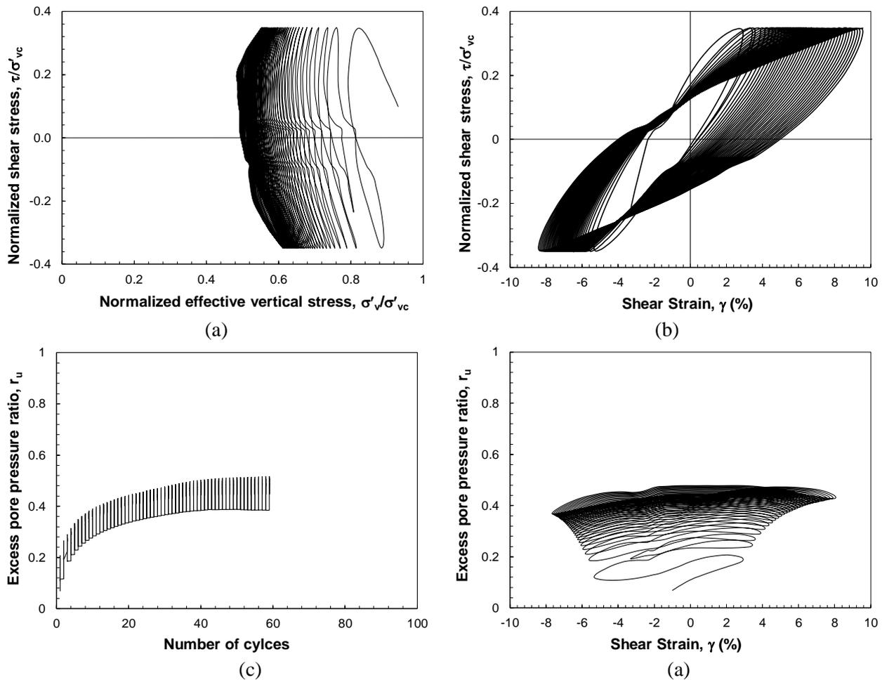
Fig. 2 - Typical results of a cyclic DSS test on Toronto peat at  $\sigma'_{vc} = 200$  kPa: (a) cyclic effective stress path, (b) cyclic shear stress-strain behavior, (c)  $r_u$  versus  $N_c$ , and (d)  $r_u$  versus  $\gamma_c$
