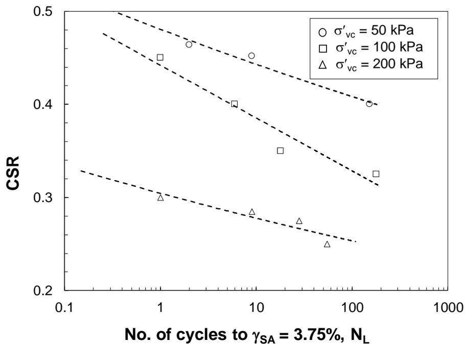
Fig. 4 - Cyclic strength curves of Toronto peat at  $\sigma'_{vc} = 50, 100, 200$  kPa
