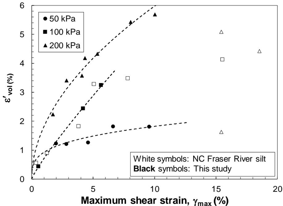
Fig. 7 - Variations of  $\varepsilon'_{vol}$  with  $\gamma_{max}$  for Toronto Peat (this study) and Fraser River silt [54] in cyclic DSS tests
