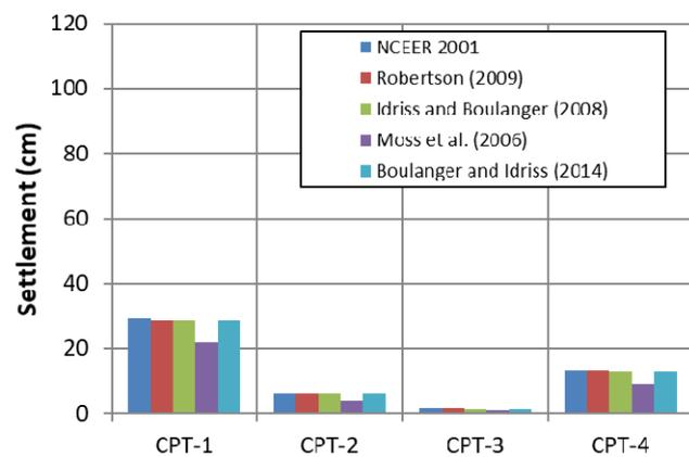
Fig. 2 – Comparison of Estimated Settlements Using Probability of Liquefaction Based Volumetric Strains from CLiq
