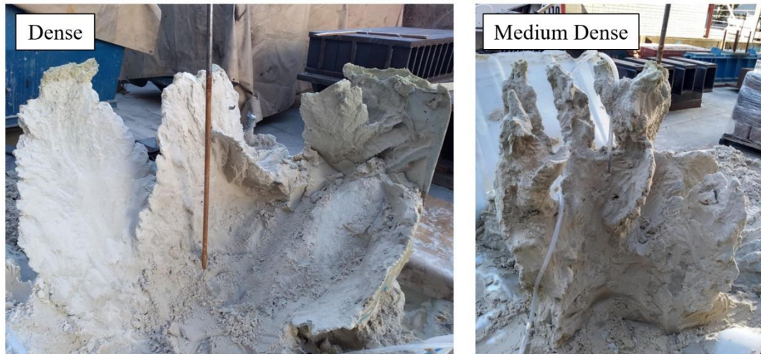
Fig. 7 – Observed composite inclusions (veins) after excavation in the dense and medium-dense specimens
