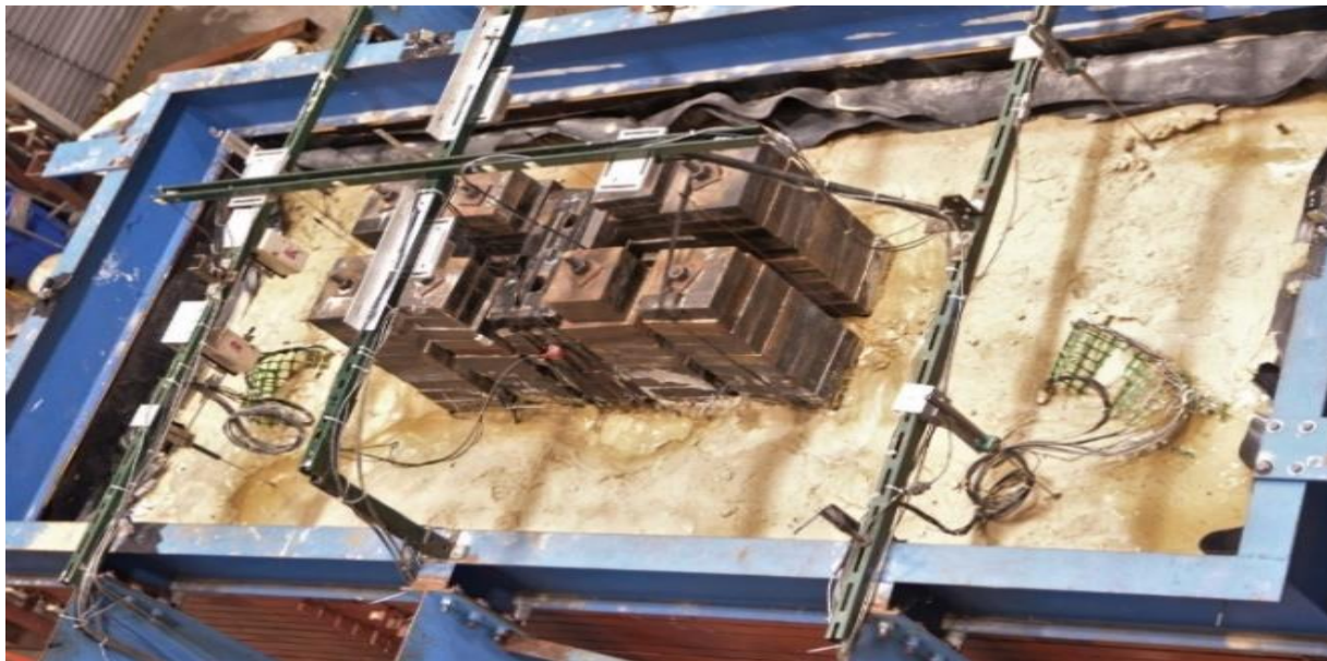
Fig. 12 – Observed soil-foundation system response after injection [21]
