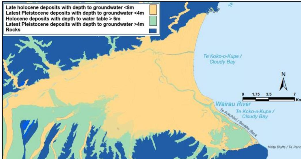
Figure 7: Geology-based liquefaction vulnerability category map for the Lower Wairau Plain
