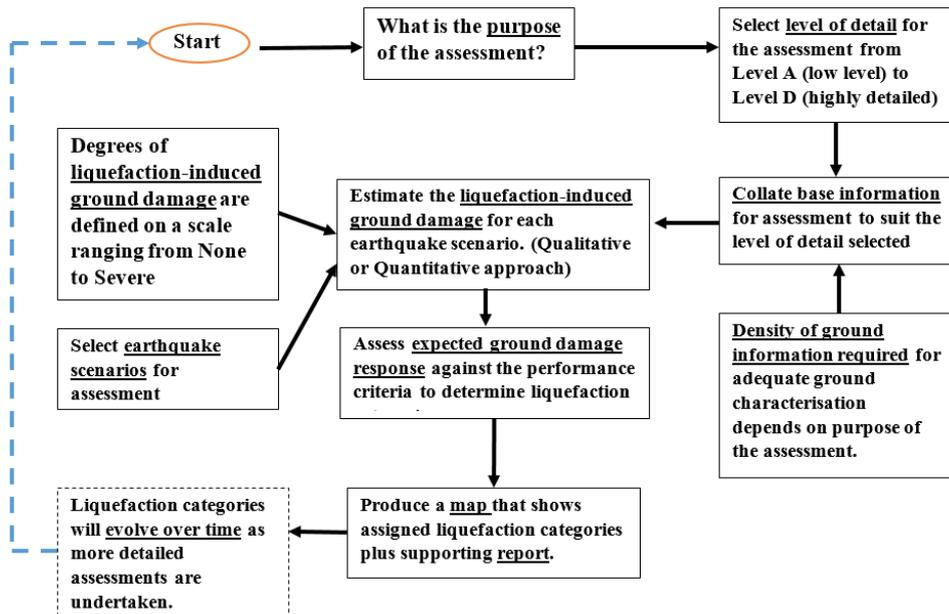
Figure 2: Overview of the recommended process for categorising the potential for liquefaction-induced ground damage [13]
