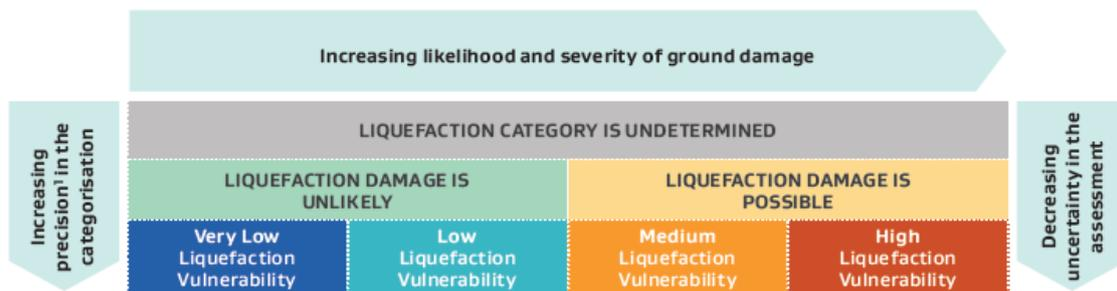
Figure 3: Recommended liquefaction vulnerability categories for use in liquefaction assessment studies to inform the planning and consenting process [13]
