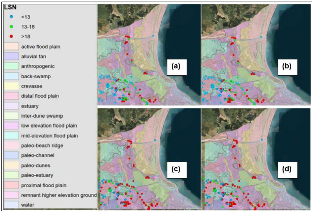
Figure 11-CPT analysis overlaid on geomorphic zones (a)  $M_w = 6.1$ ,  $PGA = 0.21g$  (b)  $M_w = 6.75$ ,  $PGA = 0.21g$  (c)  $M_w = 6.1$ ,  $PGA = 0.43g$  (d)  $M_w = 6.75$ ,  $PGA = 0.43g$
