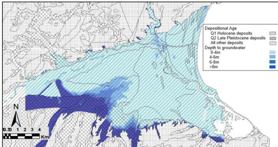
Figure 6: Depositional age of deposits and median groundwater depths for the Lower Wairau Plains
