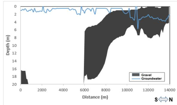
Figure 10: Location of gravel deposits and groundwater depths for cross-section NSm.
