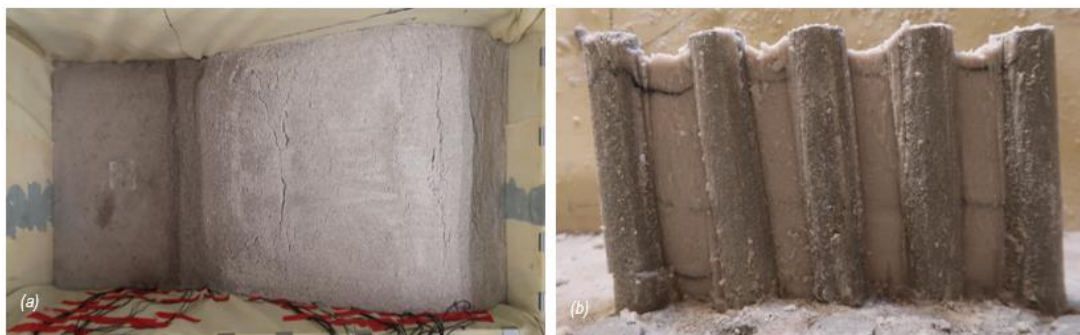
Fig. 9 – (a) Post-test photos of the embankment, and (b) Post-test excavation photos of the soil-cement columns (toe of the embankment is on the left side of photo).
