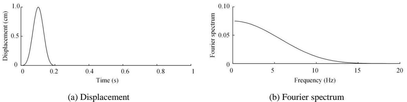
Fig. 6 – The displacement and Fourier spectrum of the incident pulse wave
