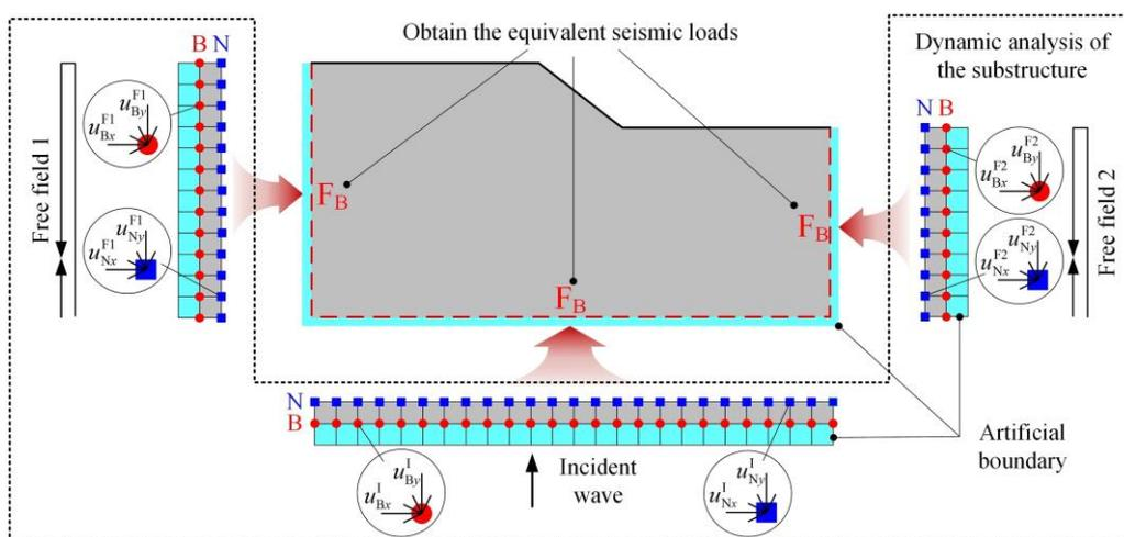
Fig. 3 – The principle and the calculation process of the hybrid wave field method: vertical incidence of seismic wave
