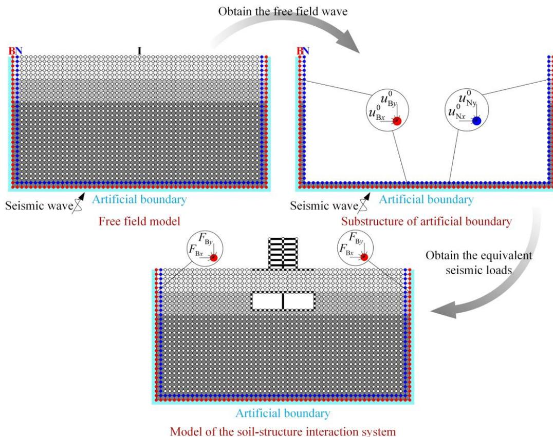
Fig. 2 –The principle and the calculation process of the boundary substructure method<sup>[10]</sup>
