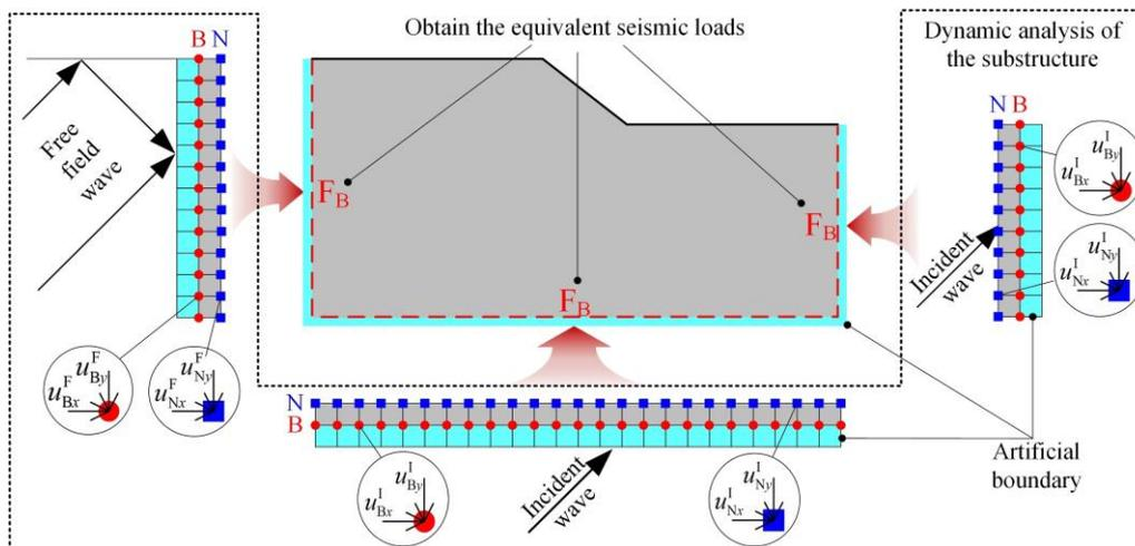
Fig. 4 – The principle and the calculation process of the hybrid wave field method: oblique incidence of seismic wave
