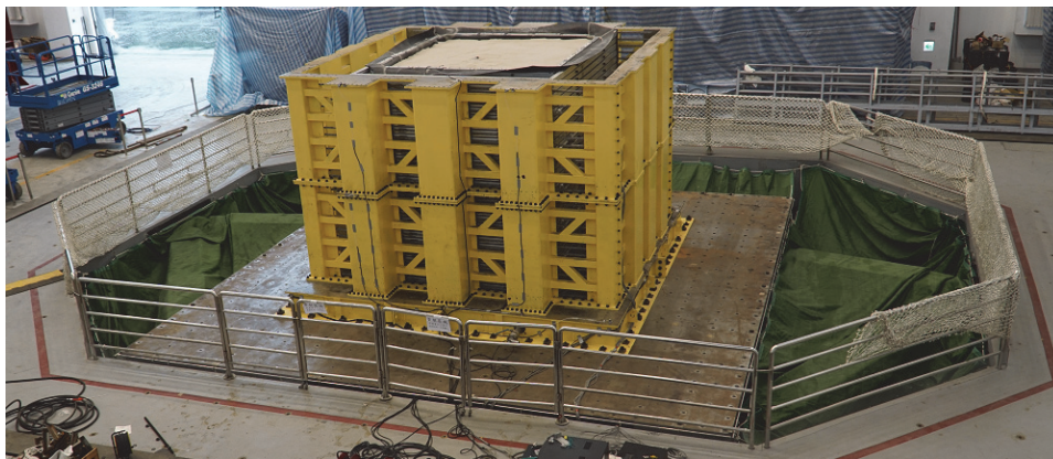
Fig. 1 – Large laminar shear box and high-performance shaking table at NCREE Tainan Laboratory
