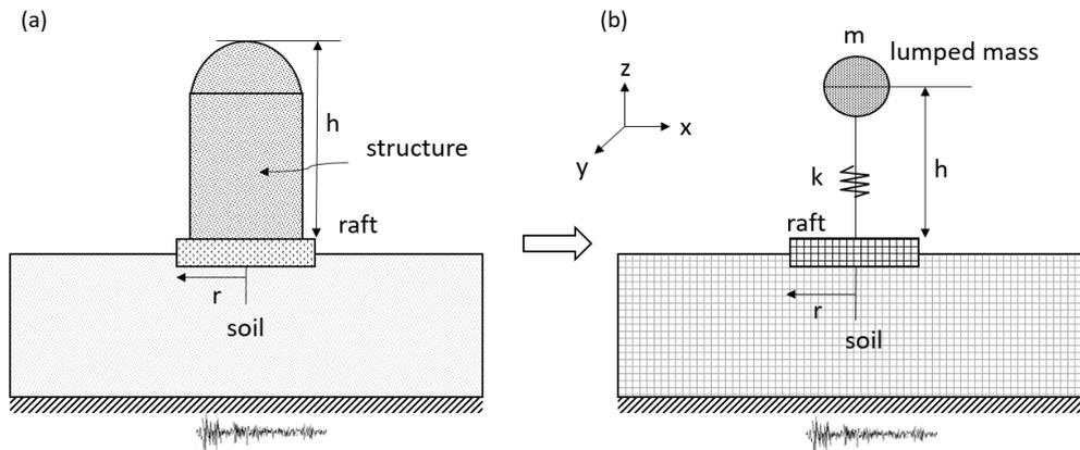
Fig. 1 – (a) Generalized NPP structure (b) Idealized finite element model of raft and soil with lumped mass model of structure
