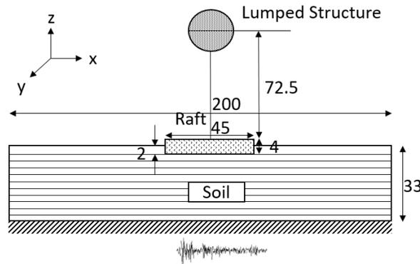
Fig. 4 – Schematic view of raft, soil and lumped structure
