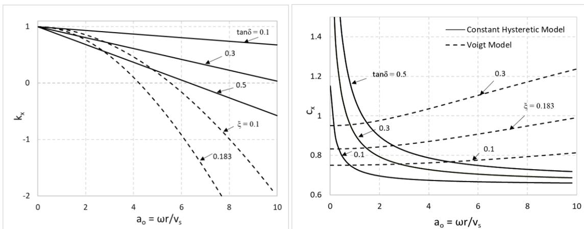
Fig. 3 – Dimensionless spring and damping coefficient in Horizontal direction, with  $\nu = 1/3$
