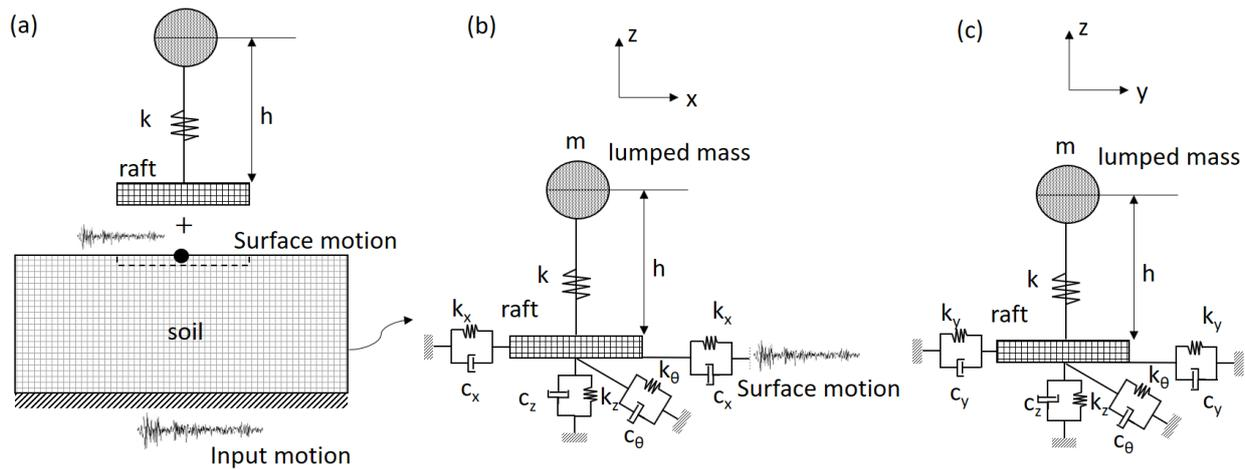
Fig. 2 – (a) Free field response, (b) Spring-dashpot model (x-z plan) and (c) Spring-dashpot model (y-z plan)
