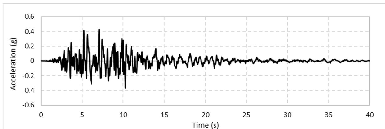
Fig. 7 – Acceleration time history at the base of raft for spring-dashpot model
