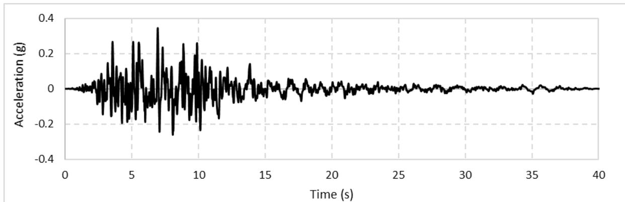
Fig. 6 – Input bedrock acceleration time history of Kobe earthquake (1995)
