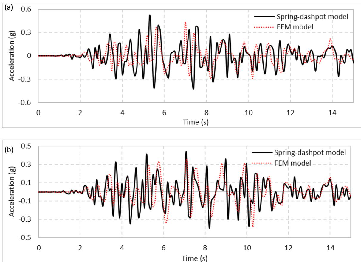
Fig. 9 – Acceleration time history at the top of structure (a) Without Embedment (b) With Embedment
