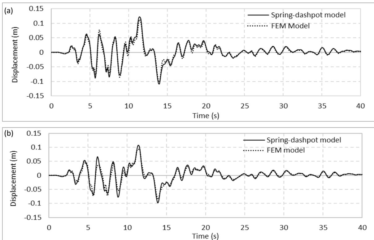
Fig. 8 – Displacement time history at the top of structure (a) Without Embedment (b) With Embedment
