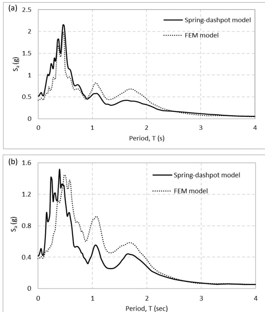
Fig. 10 – Response spectrum at the top of structure (a) Without Embedment (b) With Embedment
