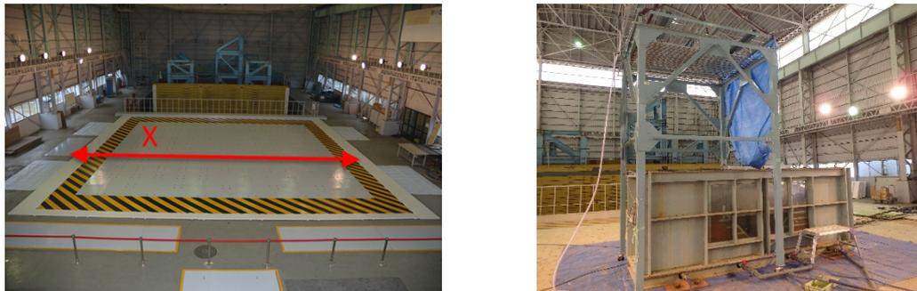
(a) Complete view of the shake table (b) Rainfall sprinkler device and soil container
