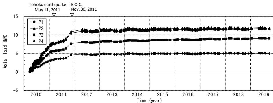
Fig. 4 – Time dependent pile head axial loads
