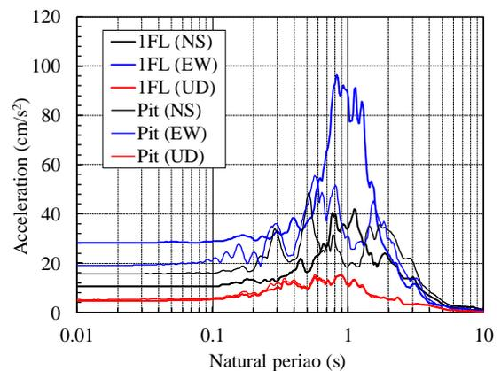
Fig. 11 – Acceleration response spectrum ( $h=5\%$ )
