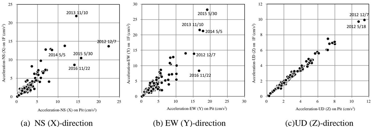
Fig. 8 – Peak accelerations on pit and 1<sup>st</sup> floor of observed seismic events
