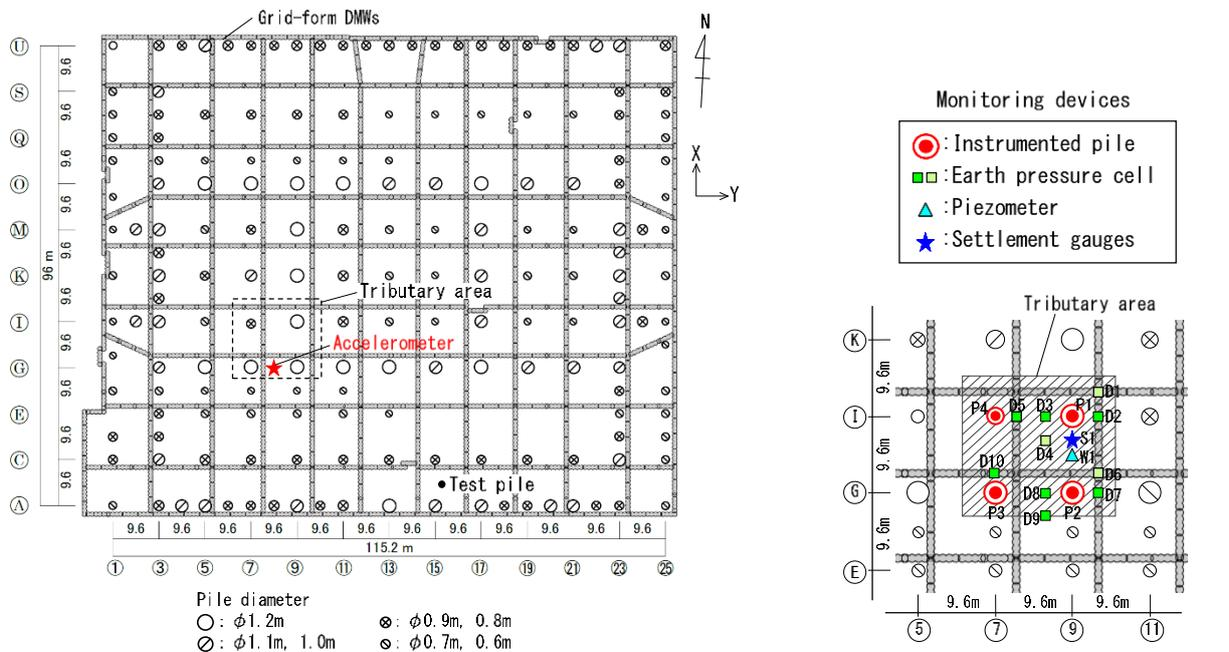
(a) Layout of piles and grid-form cement deep mixing walls
