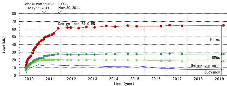
Fig. 7 – Time dependent load sharing among piles, DMWs and soil in the tributary area
