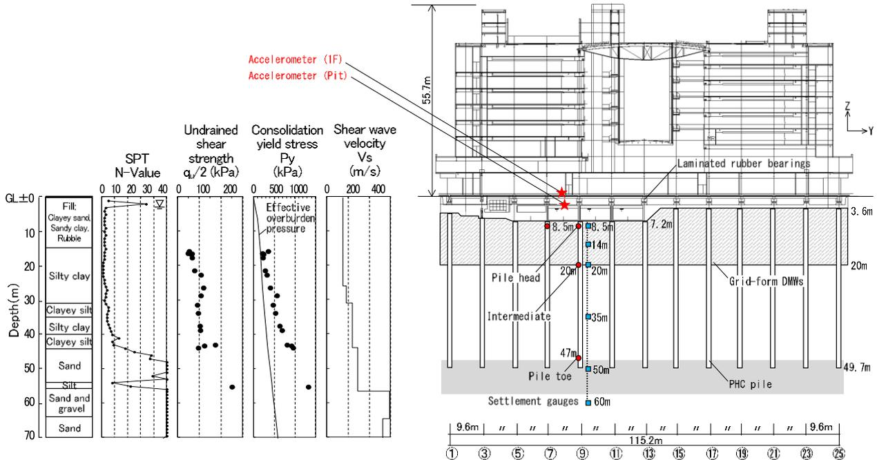
Fig. 1 – Schematic view of 12-story building and foundation with soil profile
