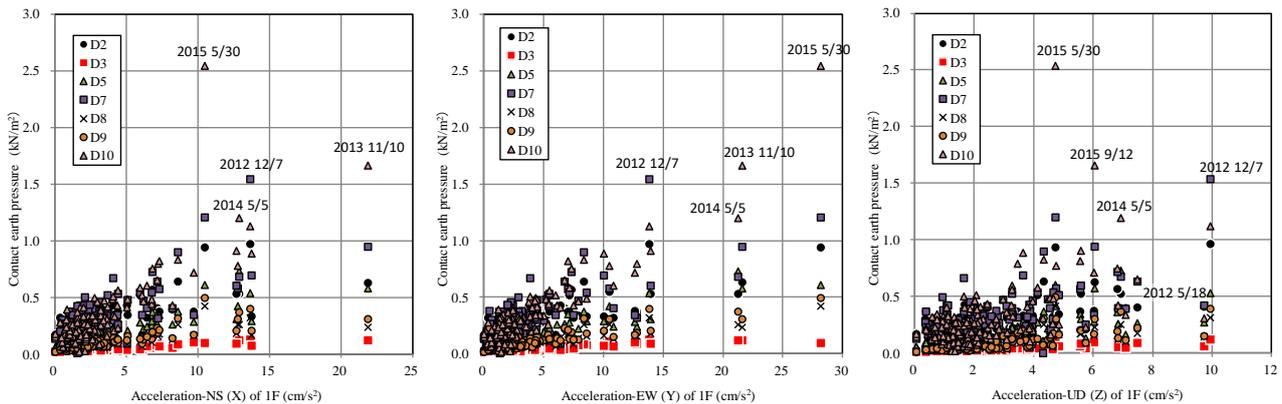
Fig. 13 – Peak contact pressures beneath the raft
