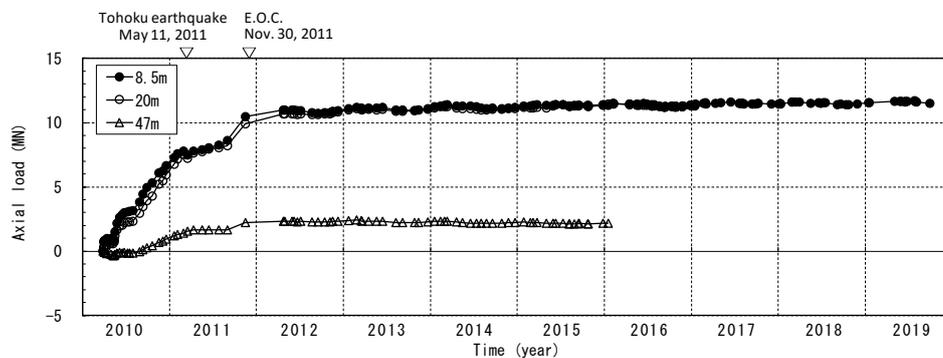
Fig. 5 – Time dependent axial loads of pile P1
