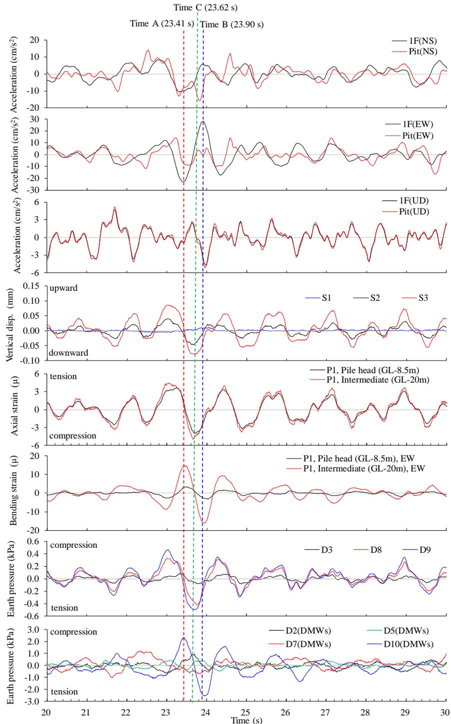
Fig. 14 – Time histories of accelerations, differential settlements, strains on piles and earth pressures during Ogasawara event (May 30, 2015)
