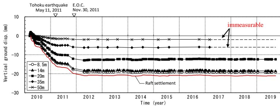
Fig. 3 – Time dependent vertical ground displacements below raft
