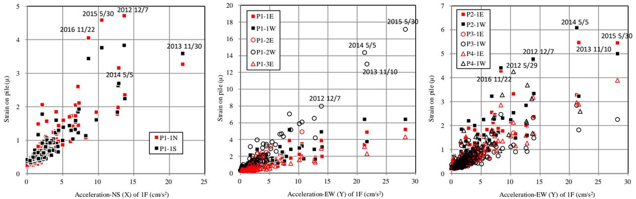
Fig. 12 – Peak strains on monitored piles
