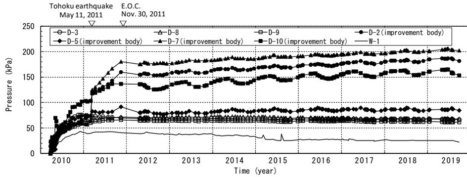
Fig. 6 – Time dependent contact earth pressure and porewater pressure
