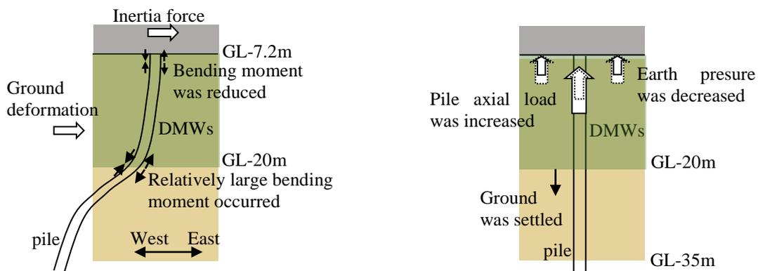
(a) Time A (at maximum inertial force of structure) (b) Time C (at maximum incremental axial load of pile)
