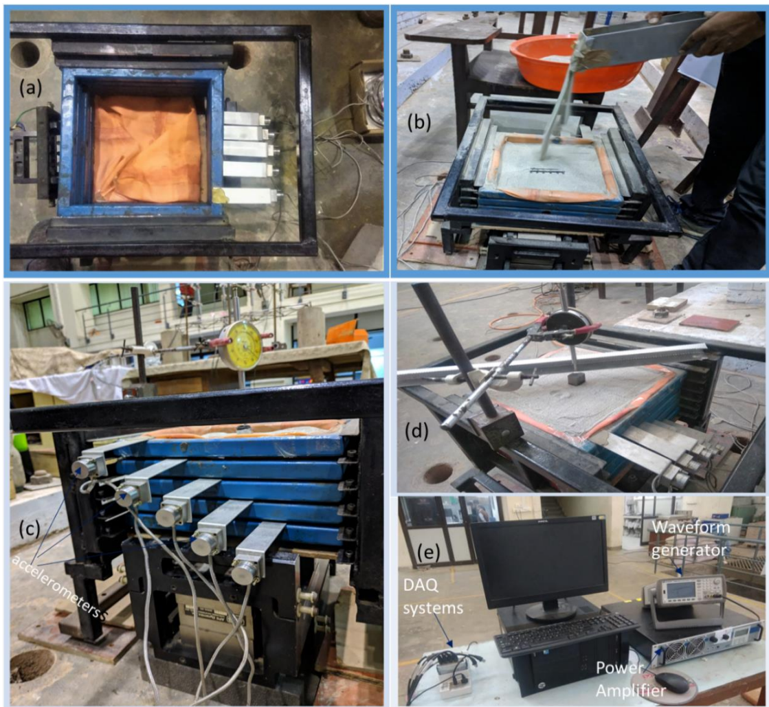
Figure 2 (a) Test setup with accelerometers and rubber membrane (b) rainfall pouring technique with geogrid maintaining the height of fall for a relative density (c) Settlement measuring dial gauge with holder and magnet on the frame (d) The aluminium light weight strip to hold the dial gauge while performing the test (e) DAQ system, Power amplifier and waveform generator to provide input frequency and acceleration amplitude into the shaker.
