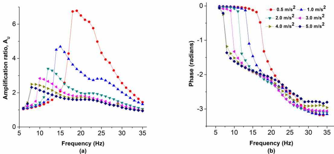
Fig. 5 – EFIM results- (a) amplification ratio and (b) phase for (Case-I).
