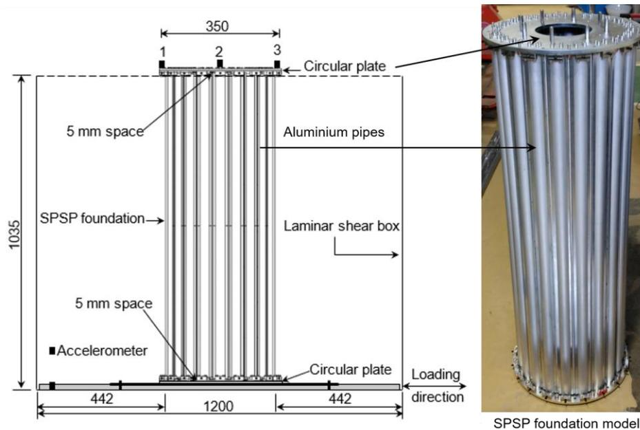
Fig. 2 – Schematic layout of experimental setup for EFIM estimation and SPSP foundation model [14].
