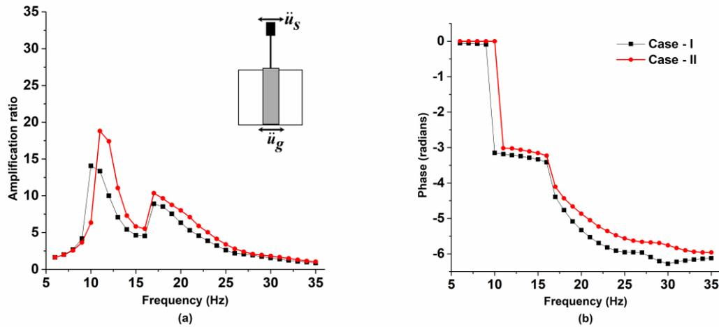
Fig. 11 – (a) Amplification ratio and (b) phase difference at the top of the superstructure for base harmonic excitation of amplitude  $1 \text{ m/s}^2$ .
