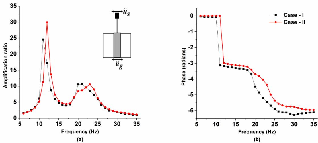
Fig. 9 – (a) Amplification ratio and (b) phase difference at the top of the superstructure for base harmonic excitation of amplitude  $0.5 \text{ m/s}^2$ .
