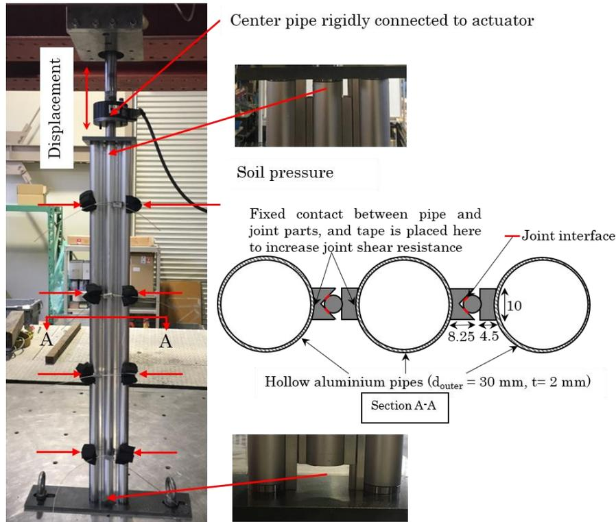
Fig. 1 – Element model of SPSP joint and joint vertical shear resistance test (all dimensions are in mm) [10].
