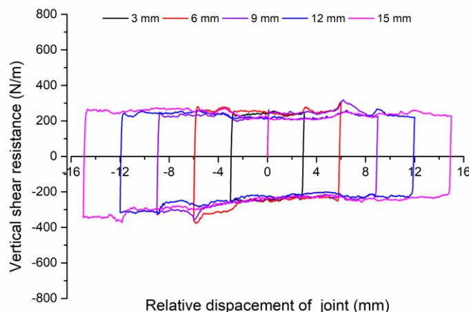
Fig. 3 – Vertical shear resistance vs relative displacement of SPSP joint (Case-a).
