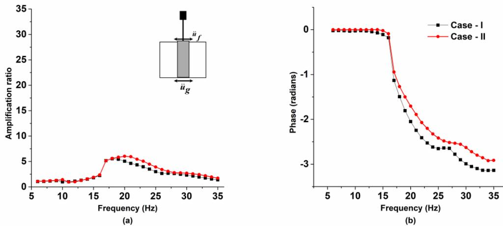
Fig. 12 – (a) Amplification ratio and (b) phase difference at the top of the footing for base harmonic excitation of amplitude  $1 \text{ m/s}^2$ .
