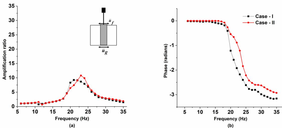
Fig. 10 – (a) Amplification ratio and (b) phase difference at the top of the footing for base harmonic excitation of amplitude  $0.5 \text{ m/s}^2$ .
