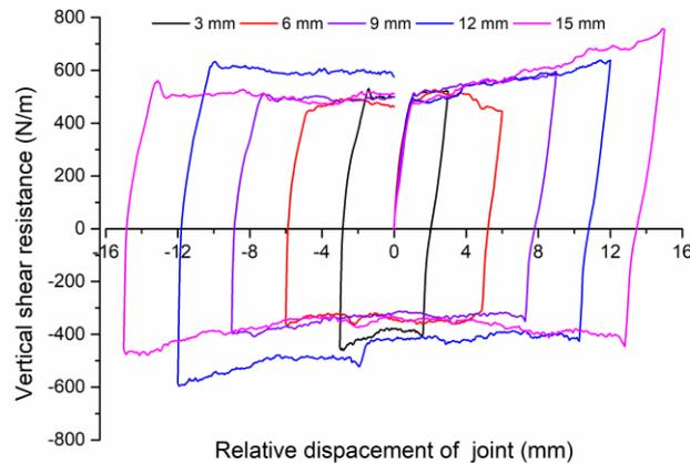
Fig. 4 – Vertical shear resistance vs relative displacement of SPSP joint (Case-b) [10].
