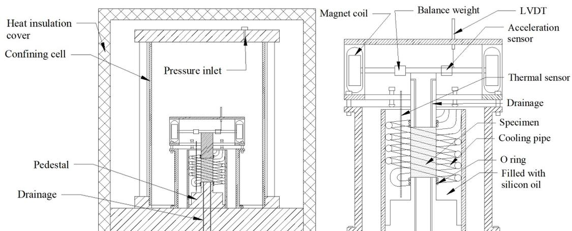
Fig. 1 –Resonant column apparatus sketch
