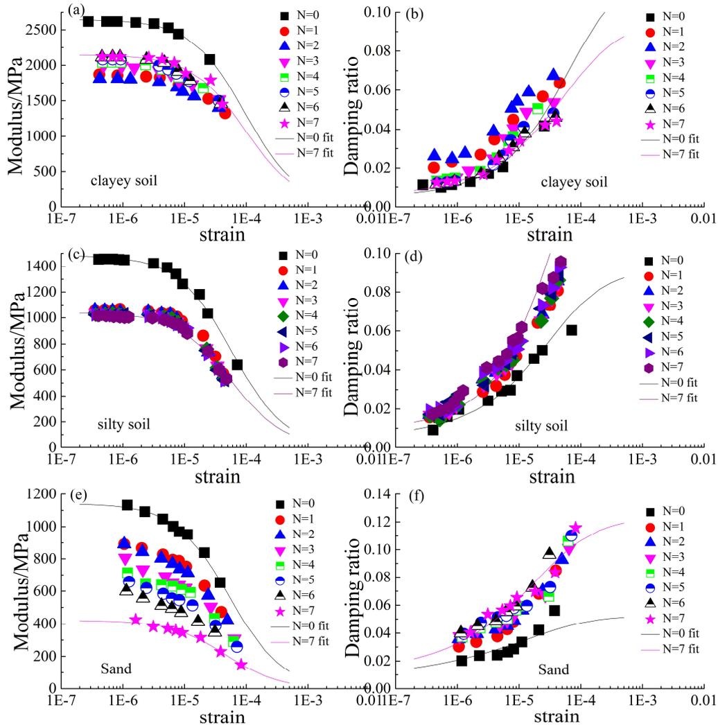
Fig. 4 –Modulus and damping ratio results of different soils
