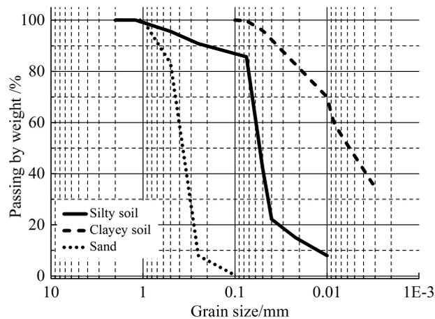
Fig. 2 – Grading curves of soils
