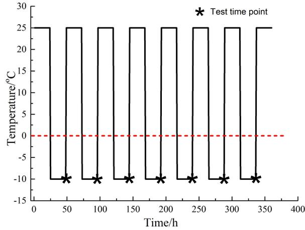
Fig. 3 –Temperature cycles for sand specimens
