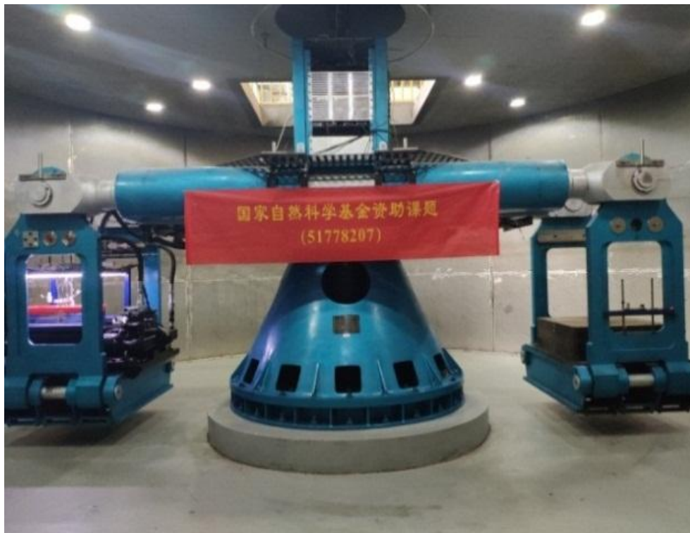
Fig. 1 – ZJU400 geotechnical centrifuge
