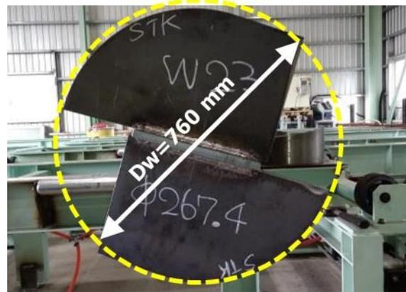
Photo 2 – Steel pipe pile with wings (W23)
