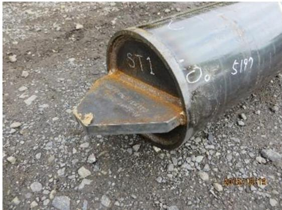
Photo 1 – Steel pipe pile without wings (ST)
