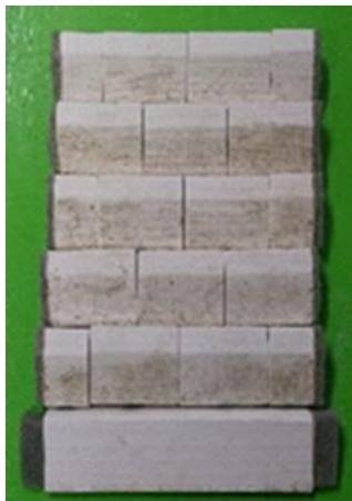
Fig.3, Retaining wall blocks on base
