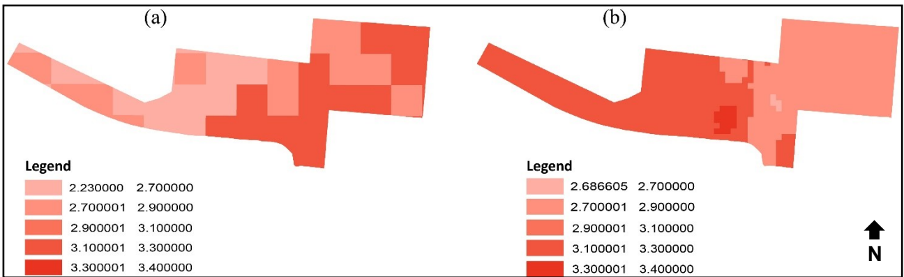
Fig. 7- Comparison of Amplification factor of Aftabnagar between (a) CDMP and (b) GSB.
