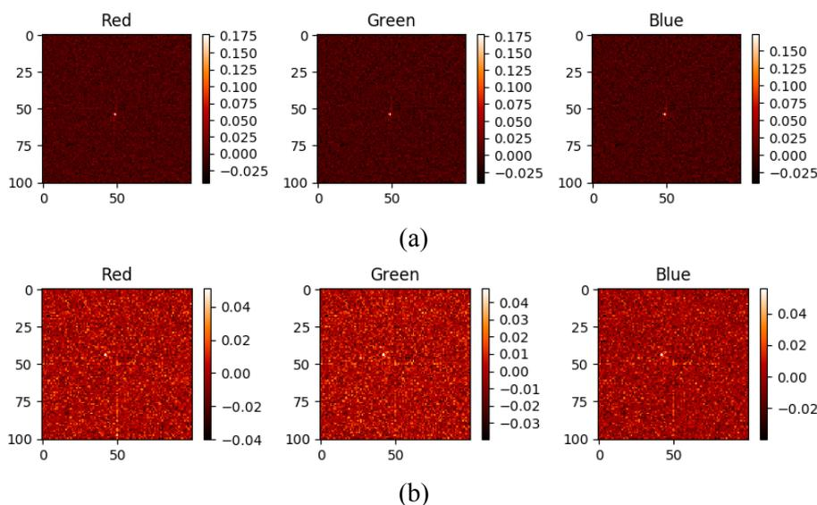
Fig. 2 – Phase correlation computed in urban areas. (a) The non-damaged urban area shown in Fig. 1a. (b) The tsunami affected urban area shown in Fig. 1b.
