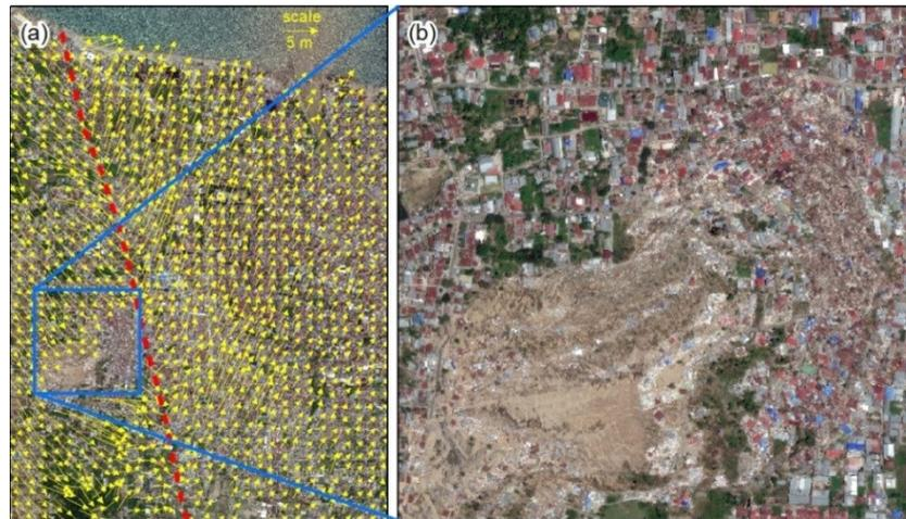
Fig. 4 – complex ground deformation at the central coast of the city of Palu, Sulawesi. (a) Coseismic displacement (yellow arrows) around the Palu-Koro fault line (dashed red line). (b) Liquefaction.
