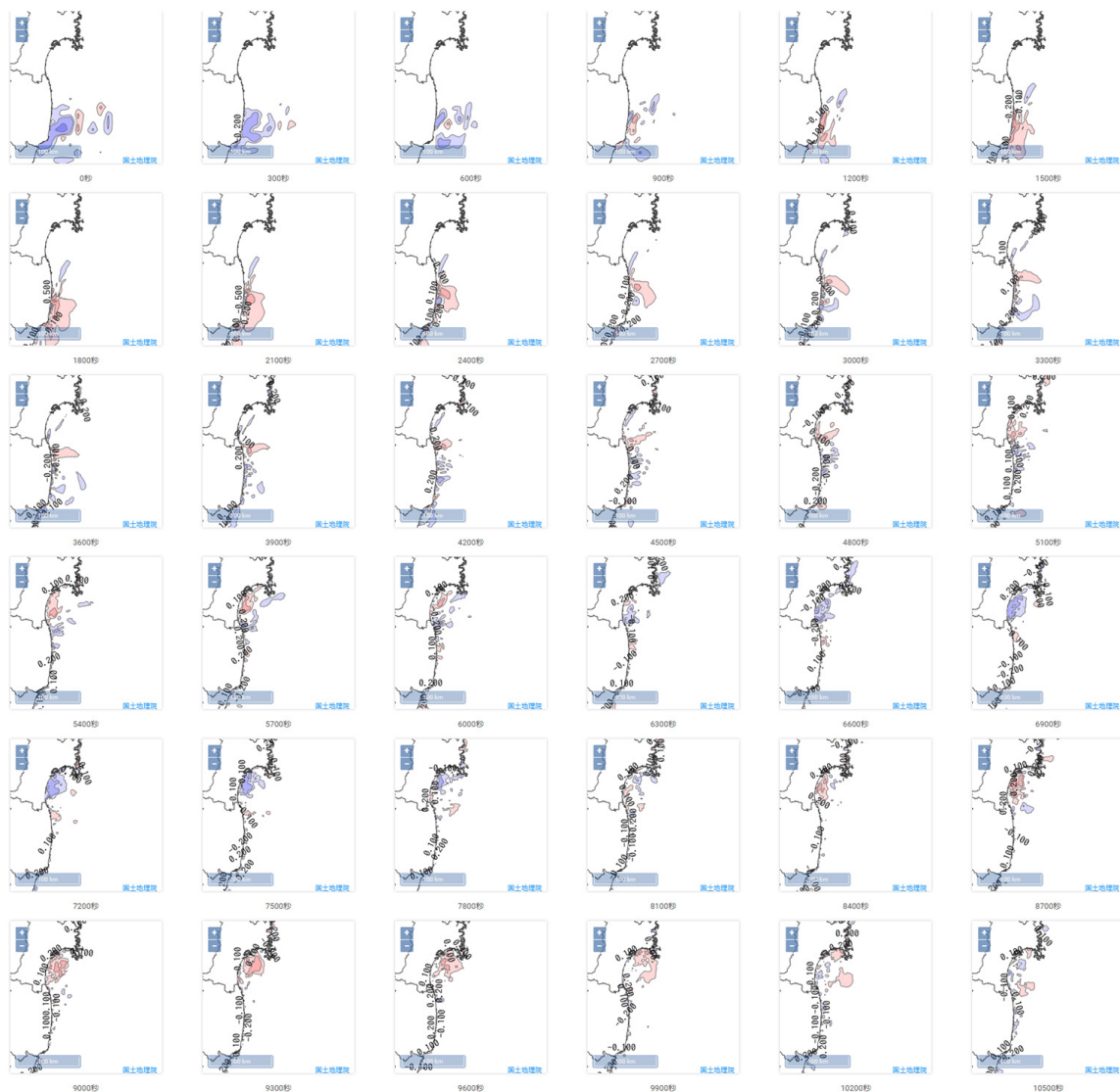
Fig. 7 – Snapshots of the forecast tsunami propagation at an interval of 300 seconds shown by the integrated visualization system
