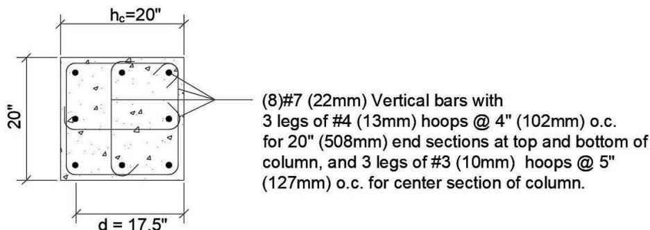
Figure 5: Original exterior gravity load column (1" = 25.4mm)
