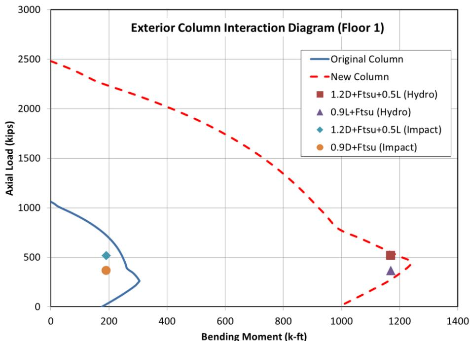
**Figure 6: Interaction diagram for typical ground floor exterior column showing tsunami load combinations for debris impact and hydrodynamic drag (1 kip = 4.45 kN; 1 k-ft = 1.36 kNm).**
