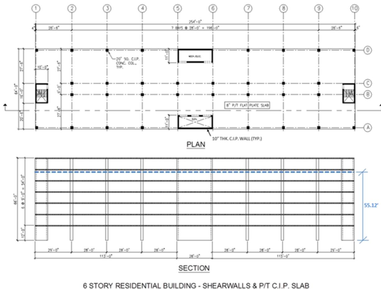
**Figure 2: Plan and section views of the prototype 7-story residential building with reinforced concrete shear walls and posttensioned flat slabs supported on gravity columns. The indicated maximum flow depth is for the Hilo, Hawaii location.**
