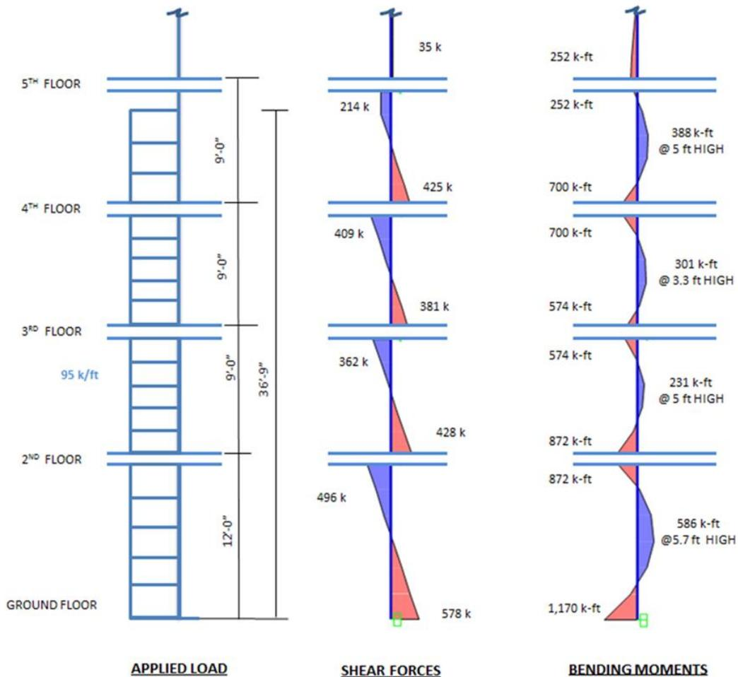
**Figure 4: Load Case 2 hydrodynamic loads on individual exterior column including the effect of debris damming (1 ft = 0.305 m; 1 k = 4.45 kN; 1 k-ft = 1.36 kNm; 1 k/ft = 14.6 kNm)**
