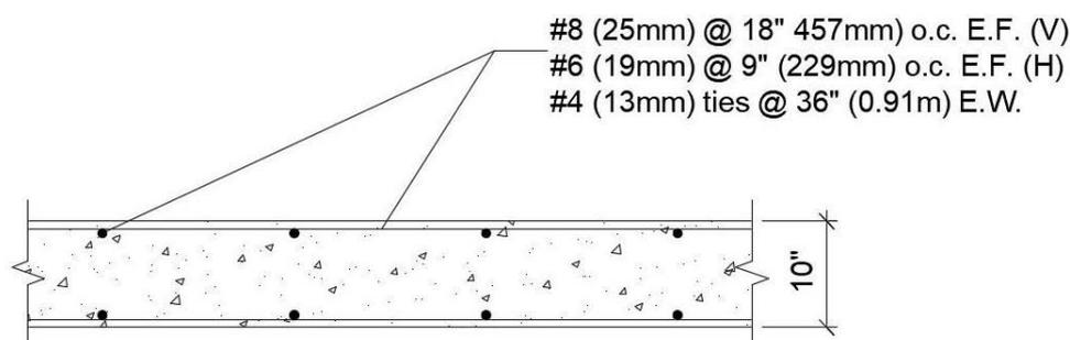
Figure 8: Original reinforcement in shear wall at ground floor (1" = 25.4mm)
