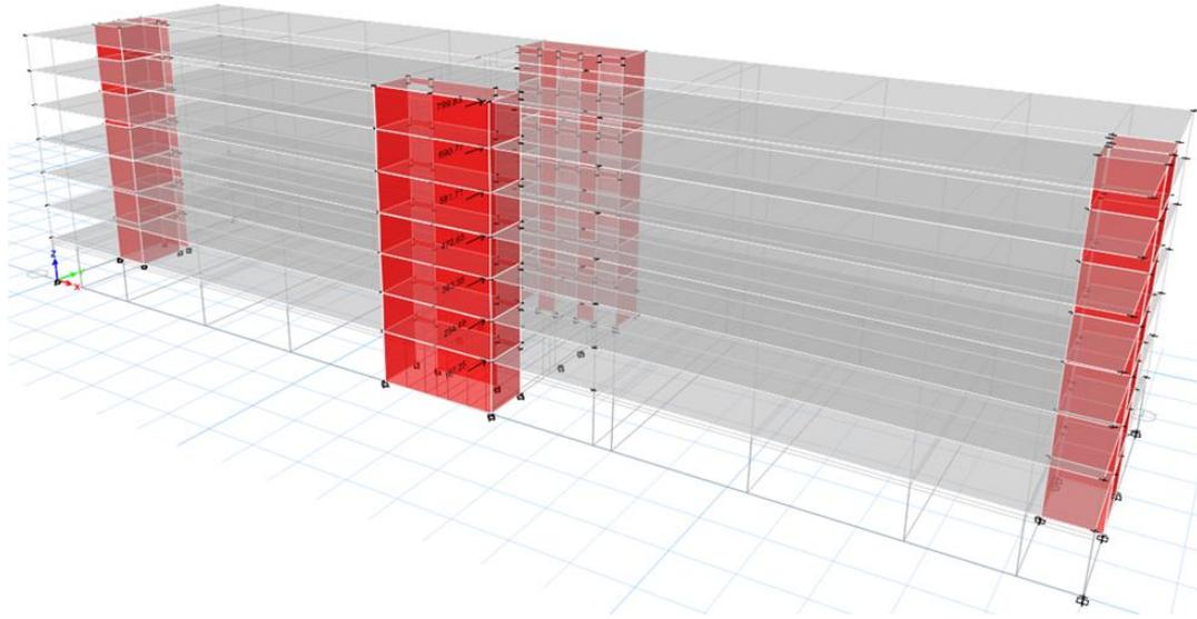
**Figure 3: ETABS computer model of residential building subjected to elevated seismic loads to meet the tsunami demand at the Hilo location**
