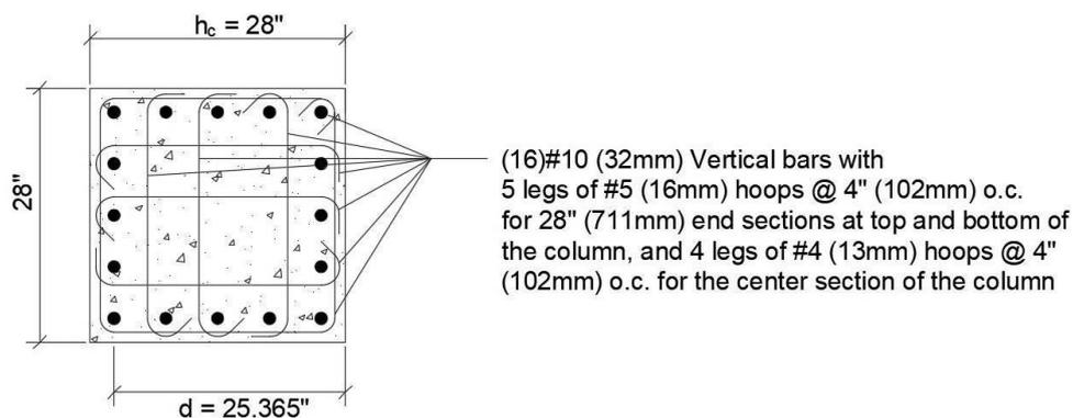
**Figure 7: Exterior first floor column including tsunami design (1" = 25.4mm)**
