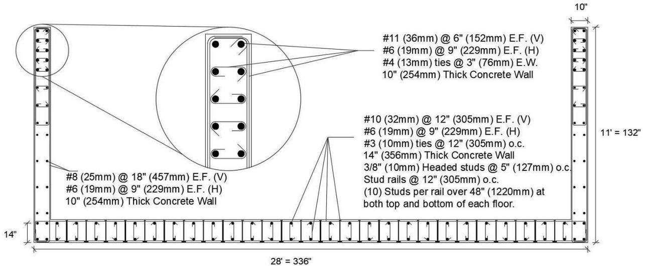
**Figure 12: New Elevator shear wall cross-section at the ground floor level**
