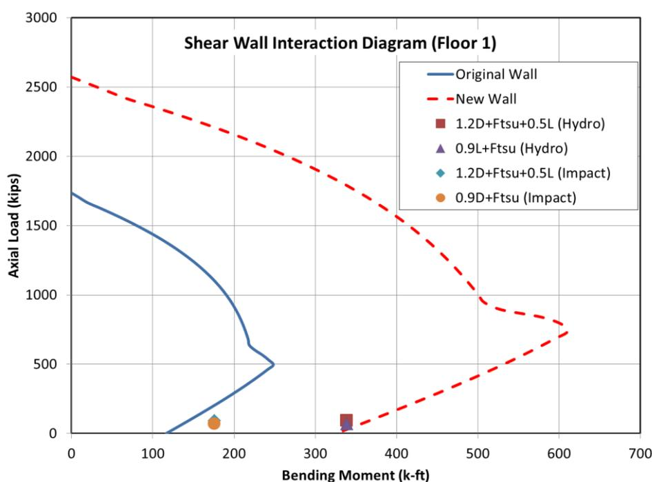
Figure 9: Interaction diagram for typical ground floor exterior wall segment showing tsunami load combinations (1 kip = 4.45 kN; 1 k-ft = 1.36 kNm).
