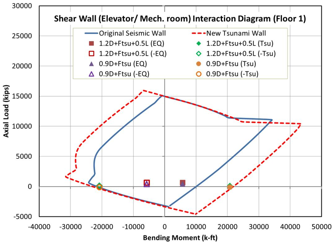
Figure 11: Interaction diagram for ground floor elevator shear wall showing seismic and tsunami load combinations (1 kip = 4.45 kN; 1 k-ft = 1.36 kNm).
