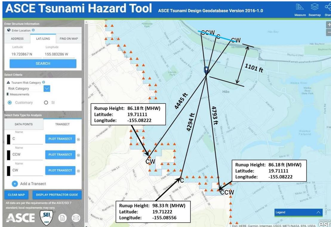
Figure 1: Hilo location for prototype building (1 ft = 0.305 m)
