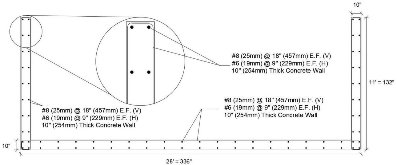
Figure 10: Original elevator shear wall cross-section at the ground floor level (1" = 25.4mm)
