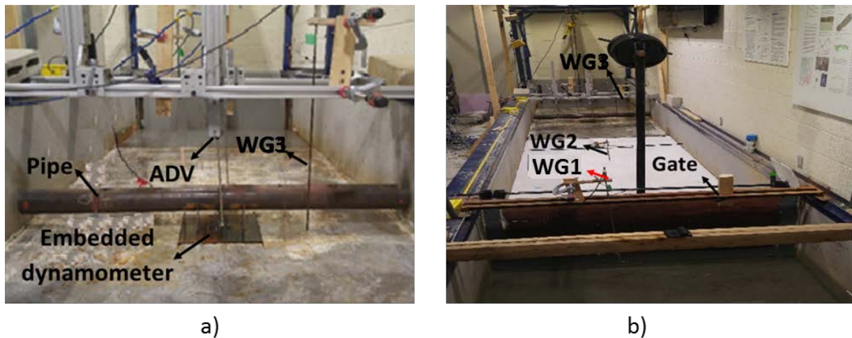
Fig. 2 - a) Downstream view, pipe, dynamometer, ADV and wave gauge, b) downstream view, gate
