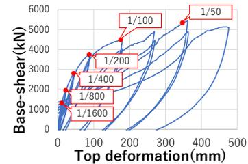
Fig.2 base shear-top deformation relationship (2014 specimen)
