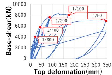
Fig.3 base shear-top deformation relationship (2015 specimen)
