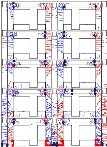
Fig. 10 damage diagram at 1/100 (2014, quote from [8])
