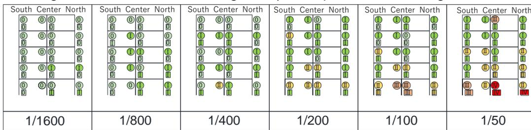
Table.4 damage state of beams(2014 specimen, ◇ : beams)
