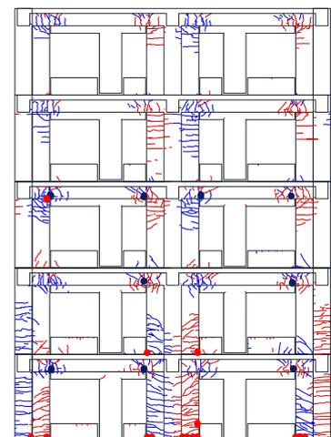
Fig.9 damage diagram at 1/200 (2014, quote from [8])
