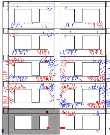
Fig. 13 damage diagram at 1/400 (2015, quote from [9])
