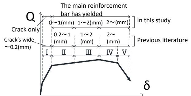
Fig.16 local damage state
