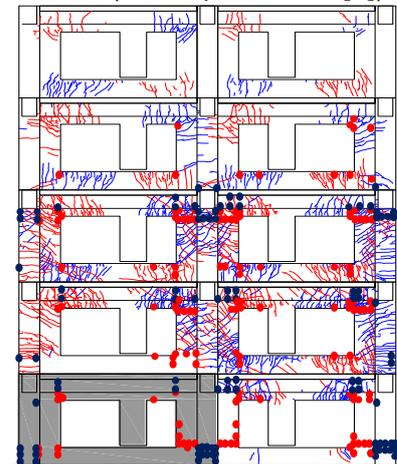
Fig. 15 damage diagram at 1/100 (2015, quote from [9])
