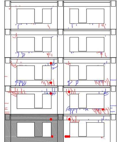
Fig. 12 damage diagram at 1/800 (2015, quote from [9])
