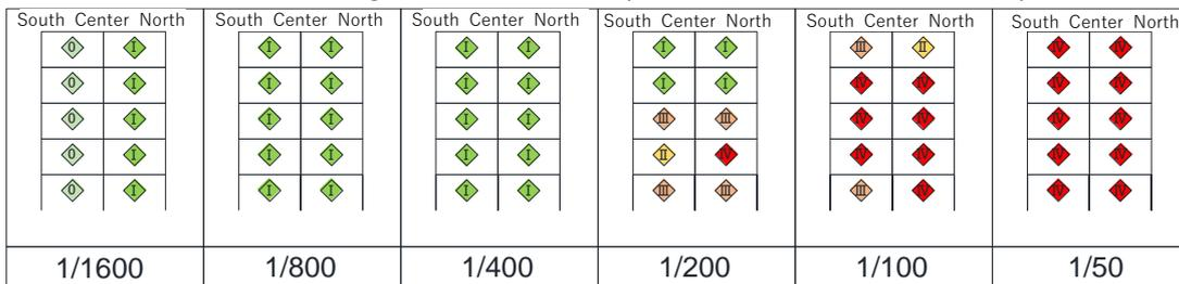
Table.5 damage state of columns and wing walls(2015 specimen, ○ : wing walls , □ : columns)
