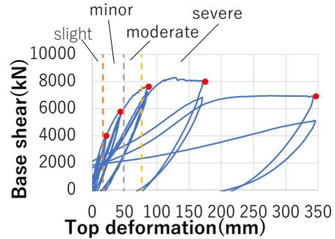
Fig.5 past global damage state (2015, wall)
