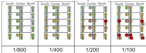
Table.6 damage state of spandrel and hanging walls.(2015, ◇ : beams, ○ : spandrel and hanging walls , ▨ : no data)
