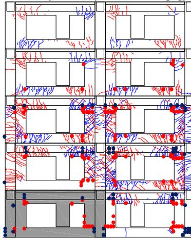
Fig. 14 damage diagram at 1/200 (2015, quote from [9])
