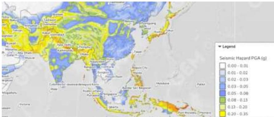
Fig. 1 – Seismic hazard maps of Central and South Asia [2]
