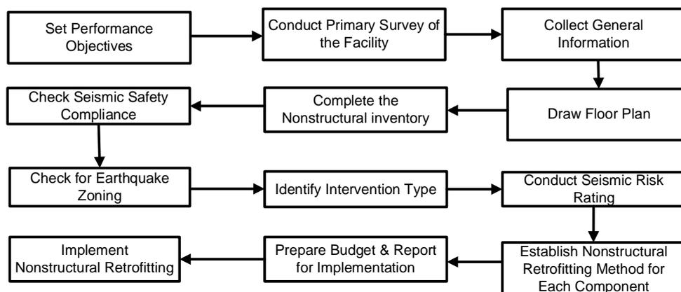
Fig. 8 – AKDN non-structural hazard mitigation approach
