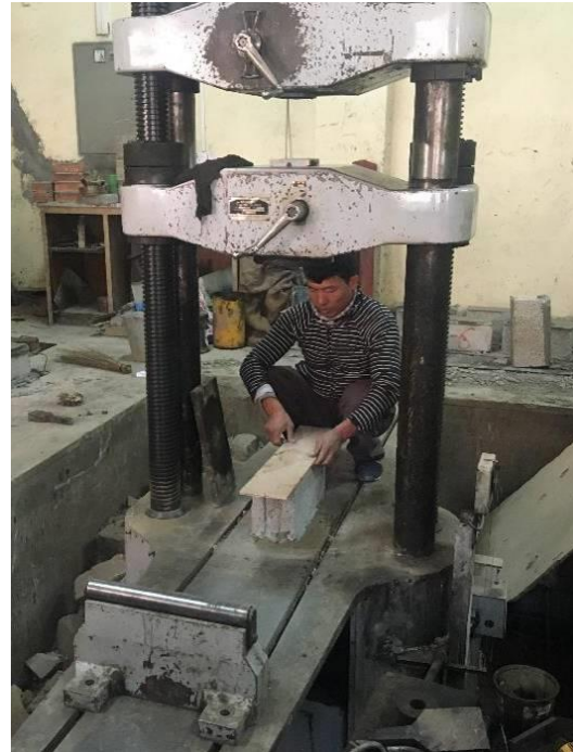
Fig. 7 – Block testing at central material testing laboratory, IoE, Tribhuvan University
