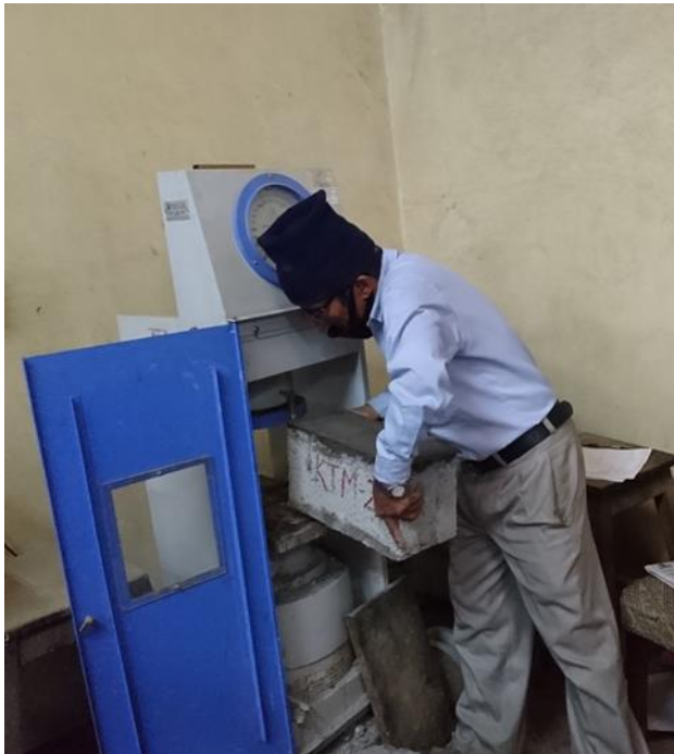
Fig. 7 – Block testing at central material testing laboratory, IoE, Tribhuvan University
