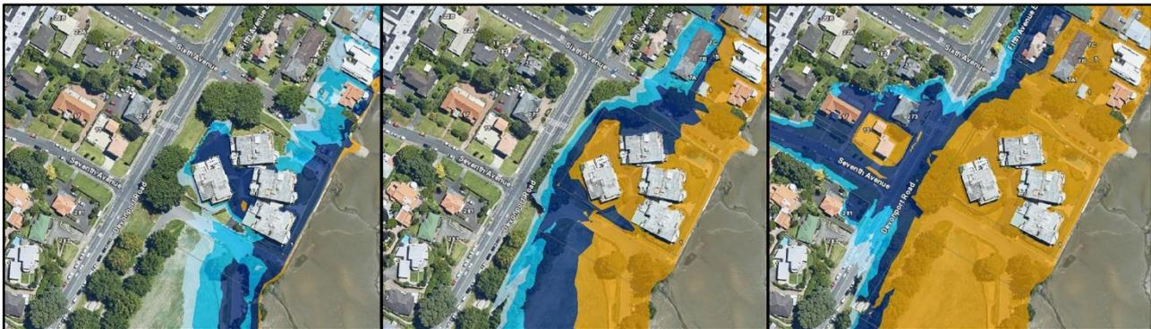
Fig. 2 - Inundation model output for 2% AEP storm 2020, 1% storm in 2080, 1% storm with 1.6mSLR 2130
