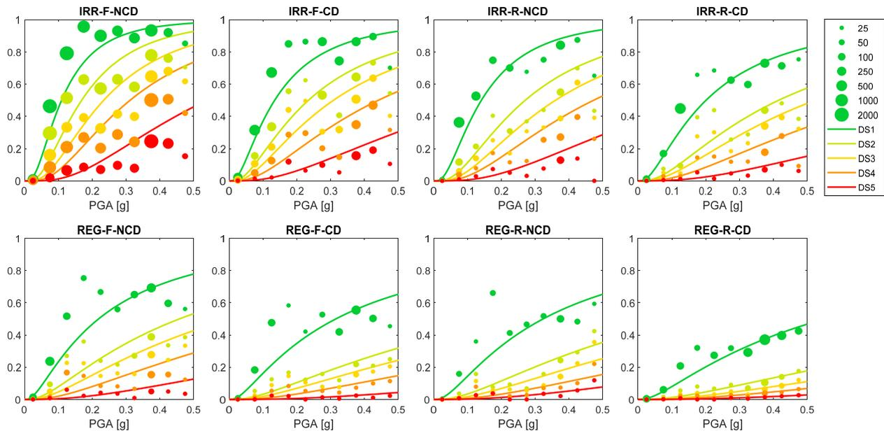
Fig. 5 – Empirical fragility curves for Italian masonry building typologies. Adapted from Rosti et al. [10]
