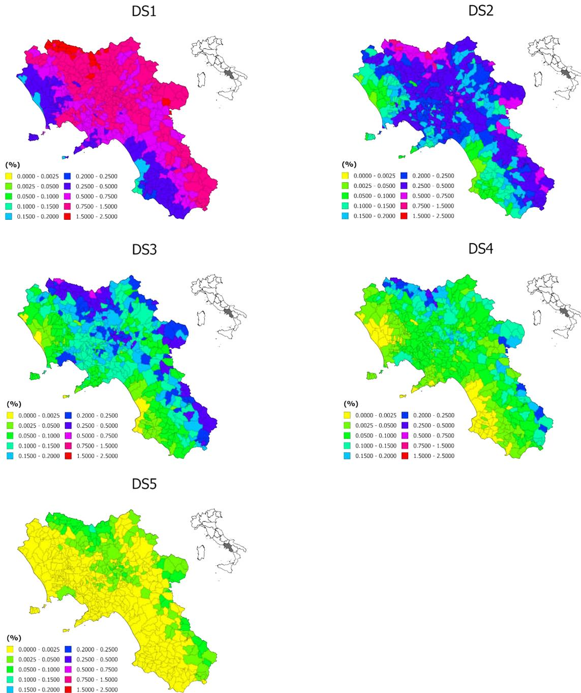
Fig. 9 – Maps of the expected percentages of masonry buildings exceeding different damage states (from D1 to DS5) in one year.
