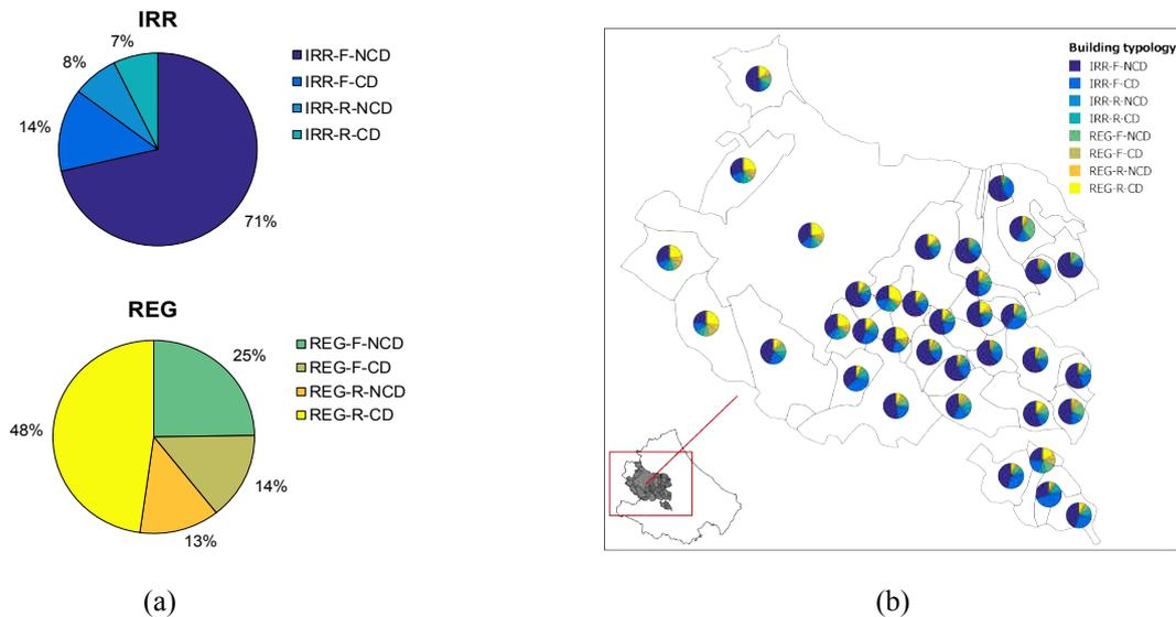
Fig. 3 – Typological classification of masonry buildings (a) and distribution of building typologies in the L'Aquila completely-surveyed municipalities (b)
