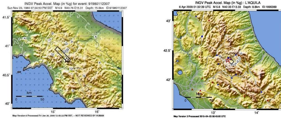
Fig. 2 – Shakemaps of the 1980 Irpinia [17] and of the 2009 L'Aquila (<http://shakemap.rm.ingv.it/shake/index.html>) seismic events
