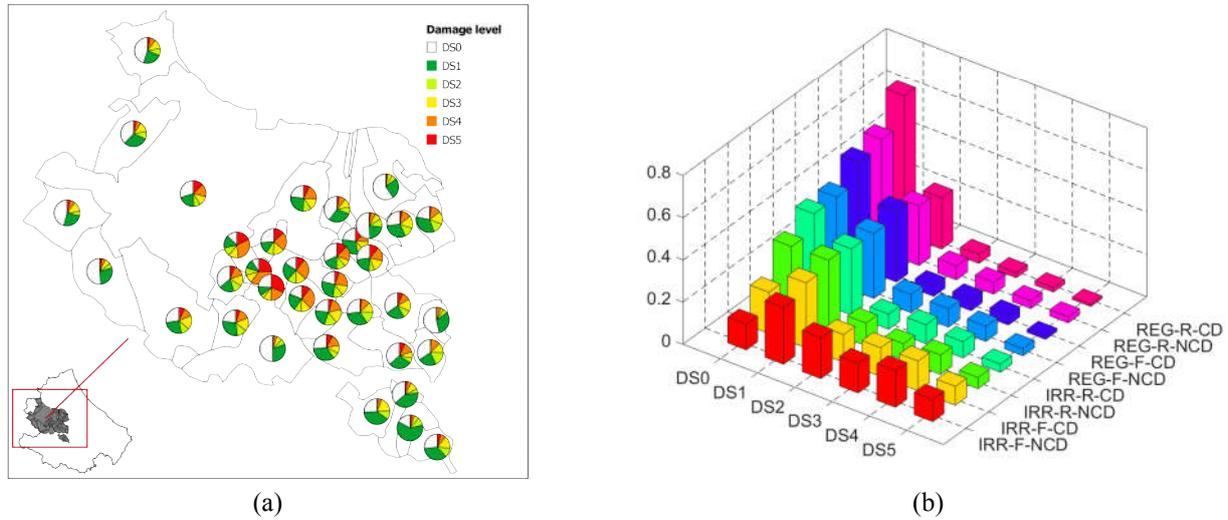
Fig. 4 – Damage distributions in the L'Aquila completely-surveyed municipalities (a) and damage distributions conditioned on building typologies (b). Adapted from Rosti et al. [10],[19].
