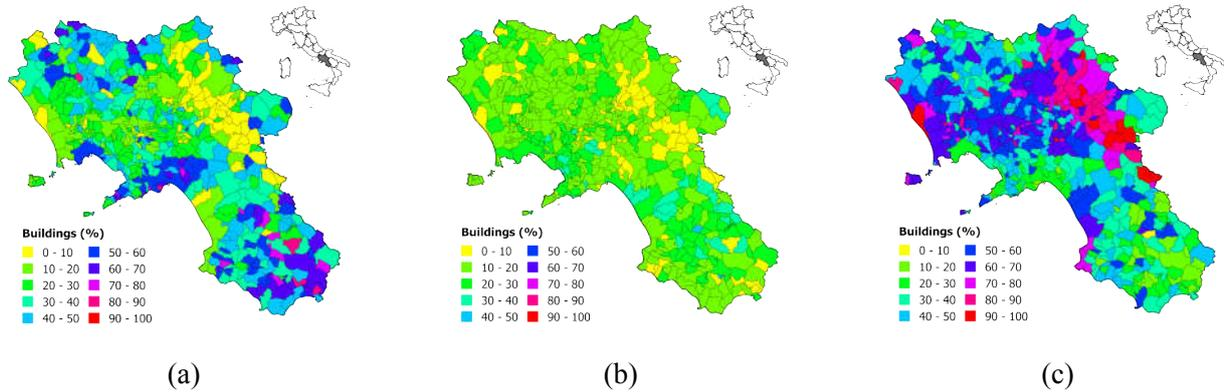
Fig. 8 – Vulnerability classification of the masonry building stock of the Campania region: percentages of masonry buildings belonging to vulnerability class A (a), B (b) and C1 (c)
