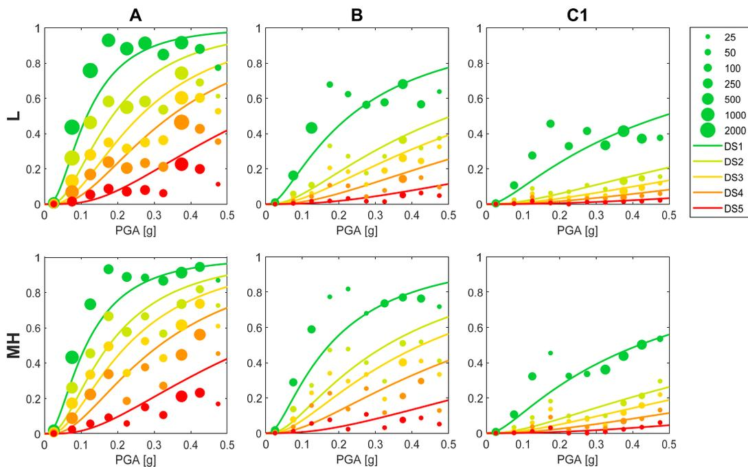
Fig. 6 – Empirical fragility curves for vulnerability classes (i.e. A: high vulnerability, B: medium vulnerability and C1: low vulnerability) and classes of building height (i.e. L: low-rise and MH: mid-/high-rise). Adapted from Rosti et al. [10]
