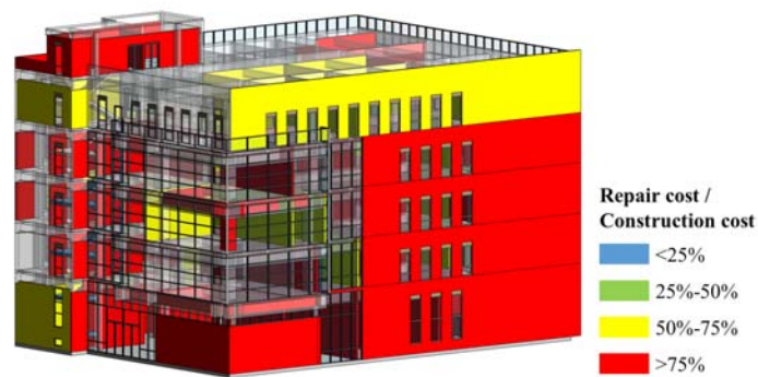
Fig. 7. Visualization of seismic losses of components [9]
