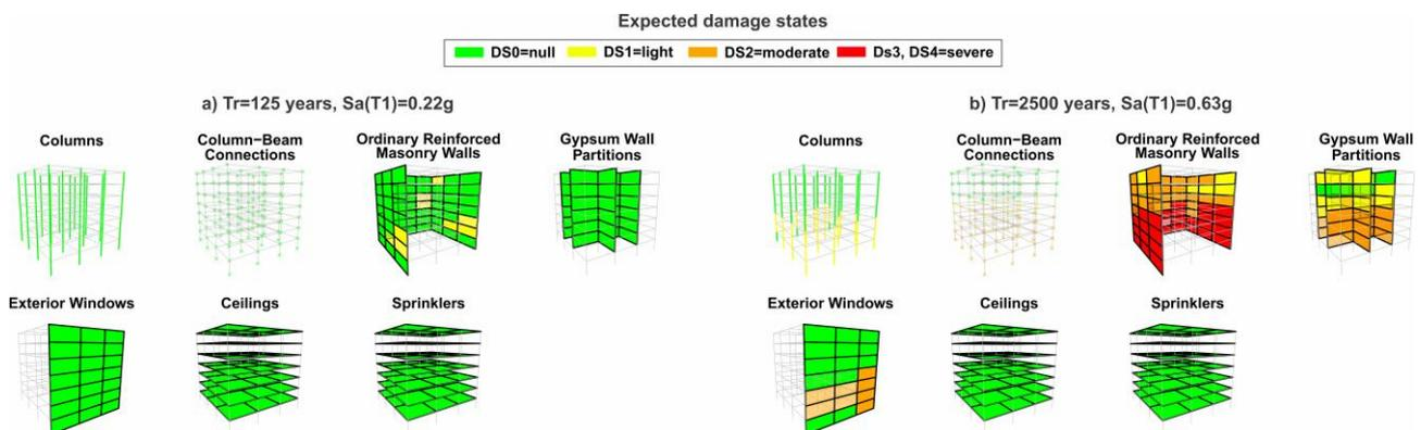
Fig. 4 – Expected damage states for the performance groups for (a) 125 and (b) 2500 years return period
