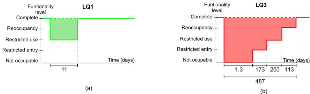
Fig. 6 – Mean recovery time for the (a) LQ1 and (b) LQ3 limit functionality states
