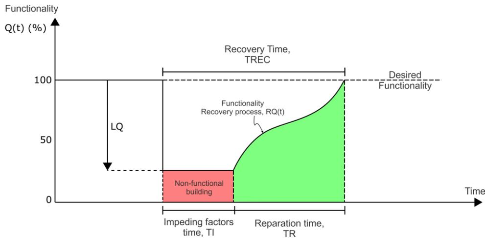
Fig. 1 – Conceptual representation of loss and recovery of functionality proposed by MCEER [2]
