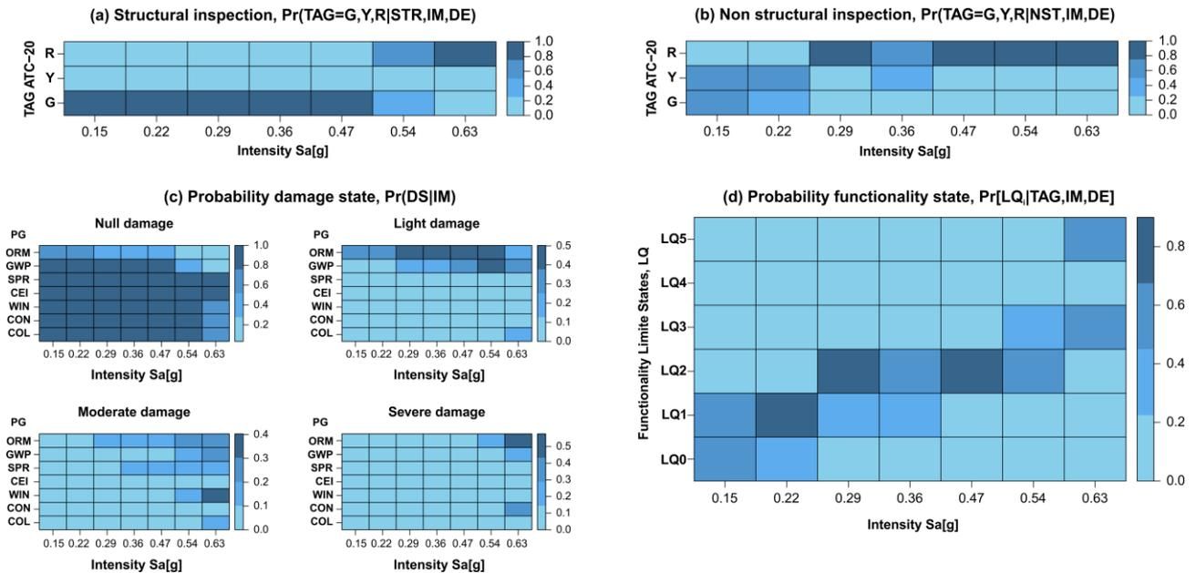
Fig. 5 – (a) and (b) probability TAGS for structural and non-structural inspection; (c) probability of damage states given a seismic intensity; (d) probability for functionality states
