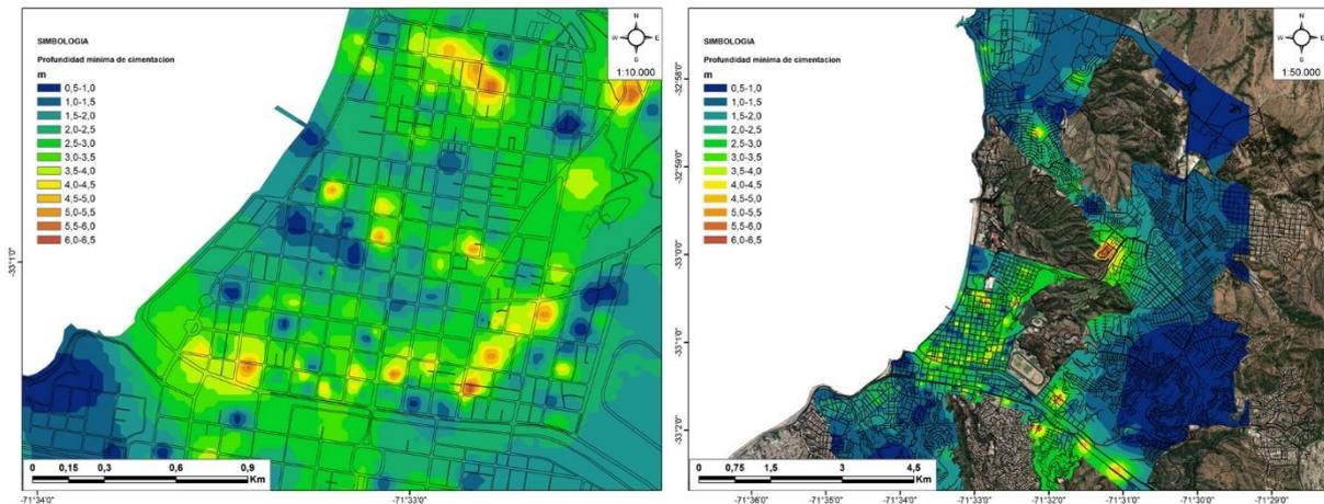
Fig. 6 – Maps of minimum foundation depth for City Plan (left) and for the entire Commune of Viña del Mar (right).
