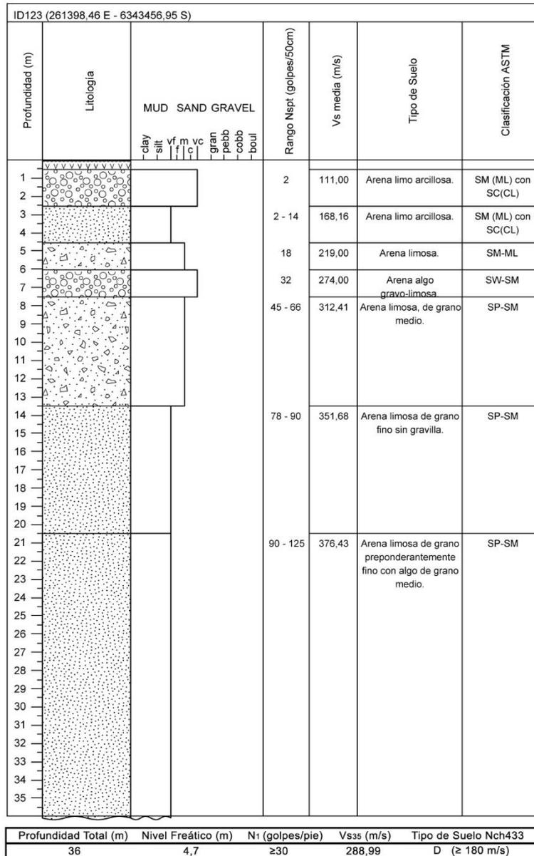
Fig. 2 – Stratigraphic column showing, every 0.5 m of survey, the lithology, size of grain, the range of NSPT as well as the average Vs per stratum, the lithological description of the soil and the USCS classification according to ASTM D2487. In addition, at the bottom of the Stratigraphic Column, a summary table is shown with the total depth of ground exploration, depth of the water table, N1, Vs<sub>35</sub> and Type of soil (from Nch433 norm).
