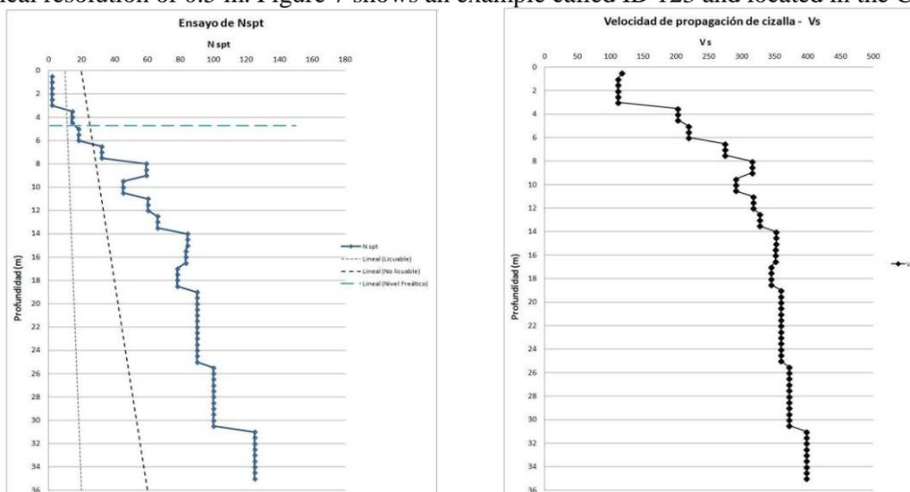
Fig. 7 – Left: NSPT versus depth graph, where the possibly liquefiable range is shown with a thin dotted line. The thickest dashed line shows the range of non-liquefiable soil and the horizontal (cyan) line the depth of the water table. Right: Graph of  $V_s$  versus depth, with increasing velocity (hardness) as the depth increases.
