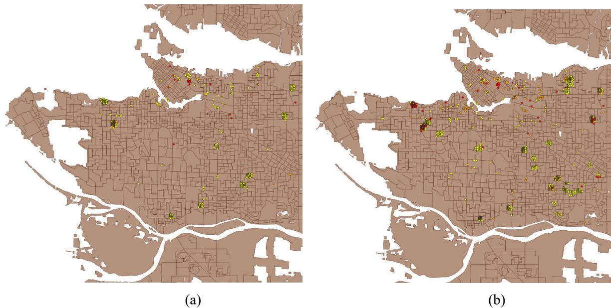
Fig. 12 - Extensive and Complete damage distribution for the CSZ9.0 Subduction Scenario using: (a) BC specific crustal fragility curves (b) BC specific subduction fragility curves
