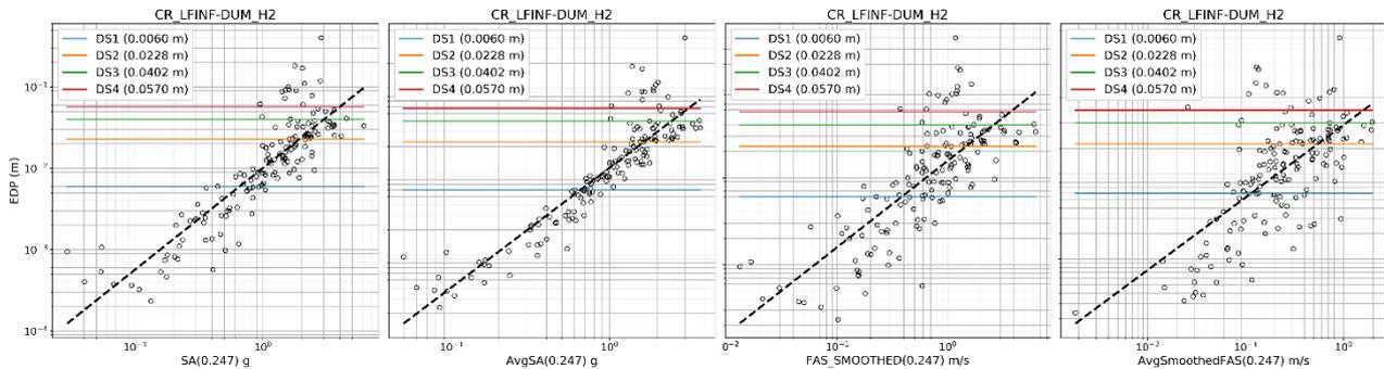
Fig. 4 – Example of linear EDP-IM models in log-log space for structural class CR/LFINF-DUM/H2 for the four IMs considered herein (in order): SA, AvgSA (0.2T – 15T), FAS, AvgFAS (0.2T – 1.5T).
