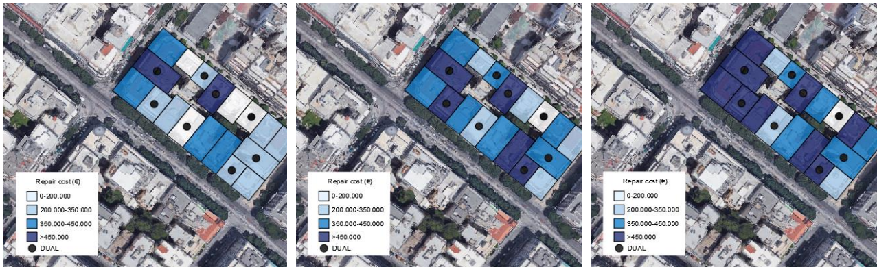
Fig. 7 – Expected spatial distribution of the repair costs (M €) of the structures under the impact of the seismic scenario with PGA=0.16g for the different soil-foundation models; Left: Fixed on rock, Middle: Fixed on nonlinear soil, Right: flexible-base nonlinear soil
