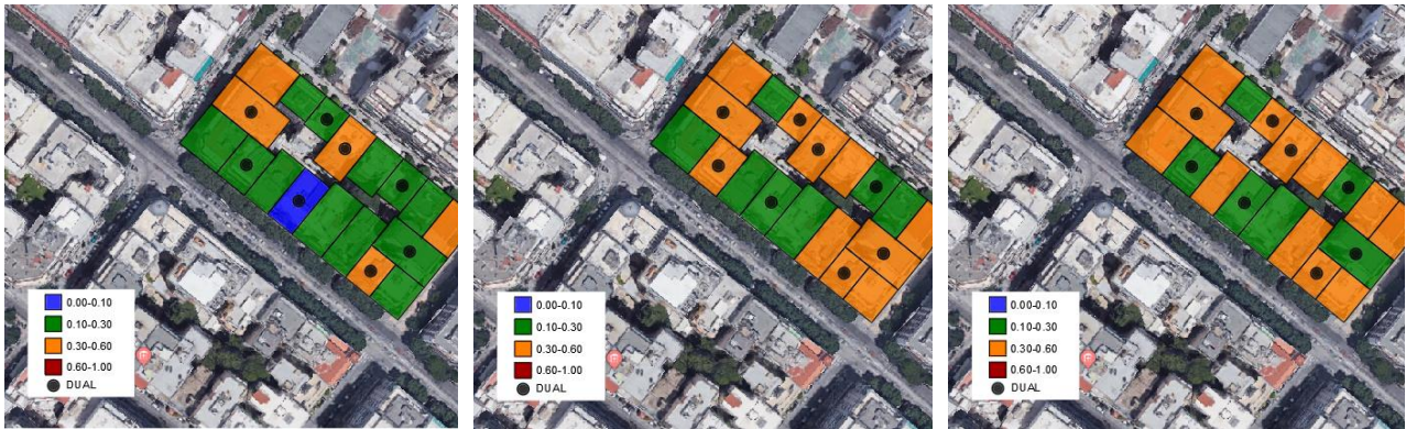
Fig. 6 – Expected spatial distribution of the losses under the impact of the seismic scenario with PGA=0.16g for the different soil-foundation models; Blue: 0-0.10 level at which construction is moderately damaged; Green: 0.10-0.30 level during which construction sustains major damage; Orange: 0.30-0.60 level at which construction is subject to severe damage; Red: 0.60-1.00, which represents the potential collapse of the structure; Left: Fixed on rock, Middle: Fixed on nonlinear soil, Right: flexible-base nonlinear soil
