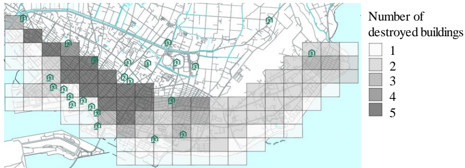
Fig.6 – Destruction distribution of buildings for earthquake
