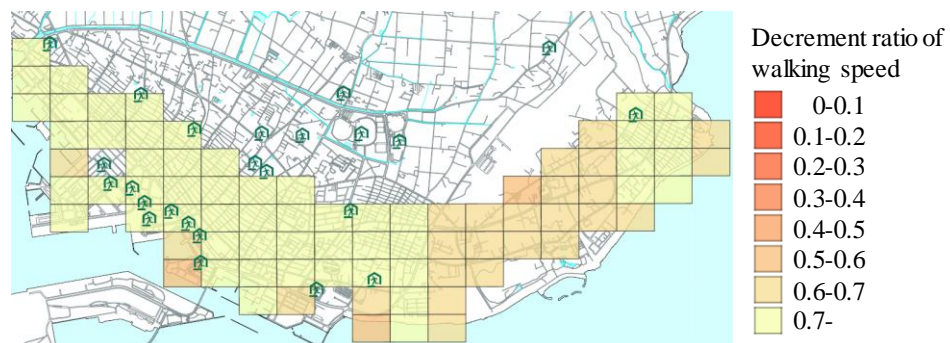
Fig.8 – Decrement ratio distribution of walking speed by street-blockade
