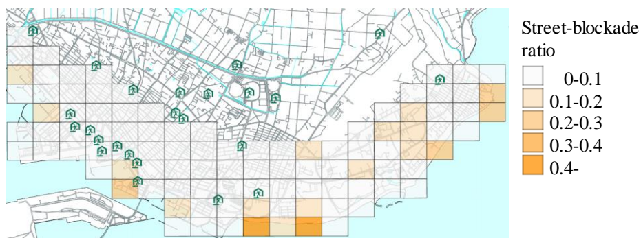
Fig.7 – Street-blockade ratio distribution by destruction of buildings
