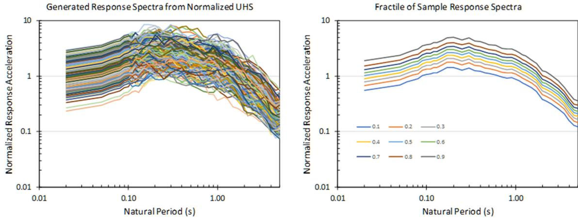
Fig. 4 – Samples of response spectra for fragility analysis.
