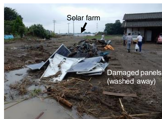
Fig. 13– Example of damage to solar farm (2015 Kanto flood, Japan)
