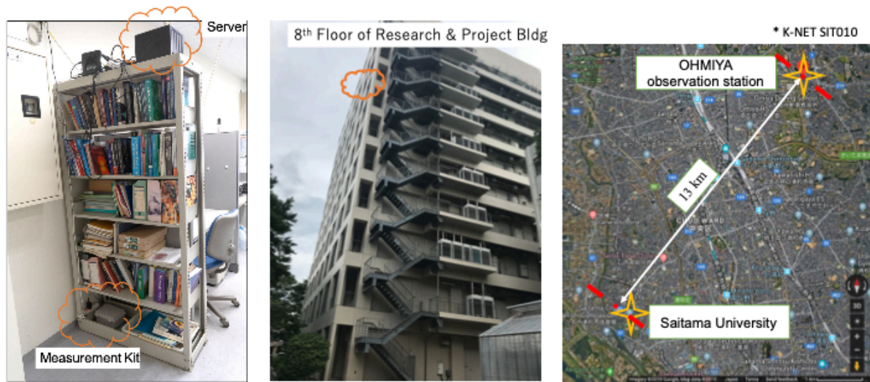
Fig. 10 – Deploying the IoT sensing SSM in a 10 Floor Building
