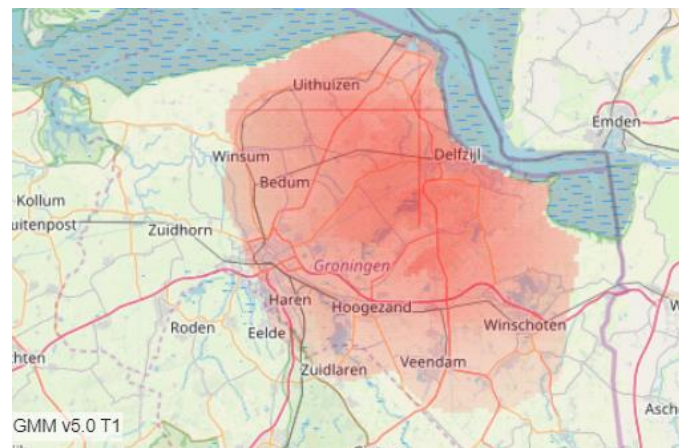
(b) Seismicity in Groningen, The Netherlands caused by natural gas extraction.
