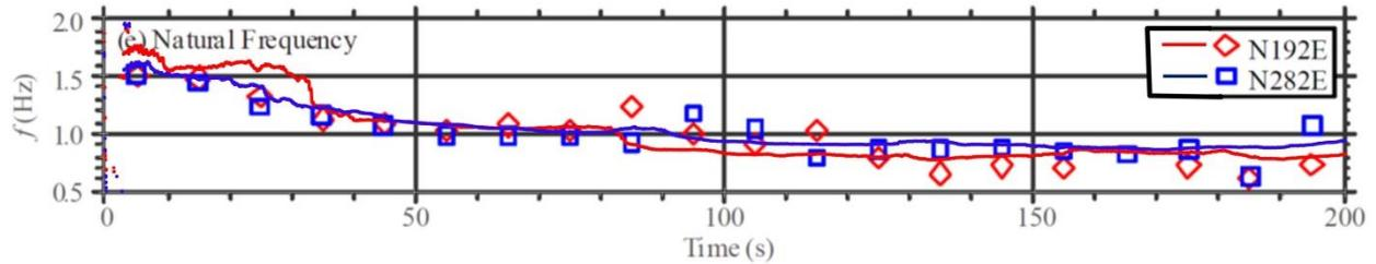
Fig. 3 – Comparison of the estimated natural frequencies; derived natural frequency from the C method is overlaid as blue and red lines on the identified natural frequencies by BRI [2] as square and diamond marks.
