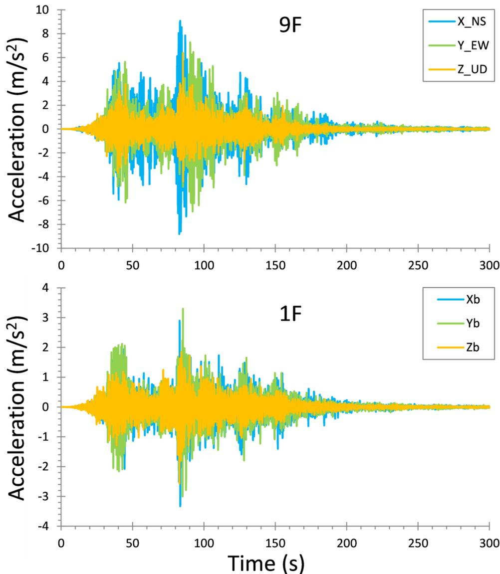
Fig. 2 – Accelerogram of the 311 Earthquake observed at 9F and 1F of Civil Engineering and Architecture Research Building of Tohoku University
