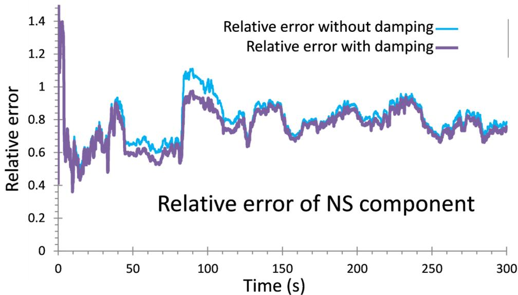
Fig. 6 – Change of the relative error for the NS component of 1F derived from the waveform at 9F applying the C method
