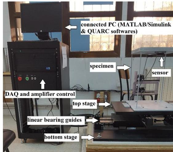
Fig. 1 – Experimental setup of the electric linear motor bi-axial shaking table
