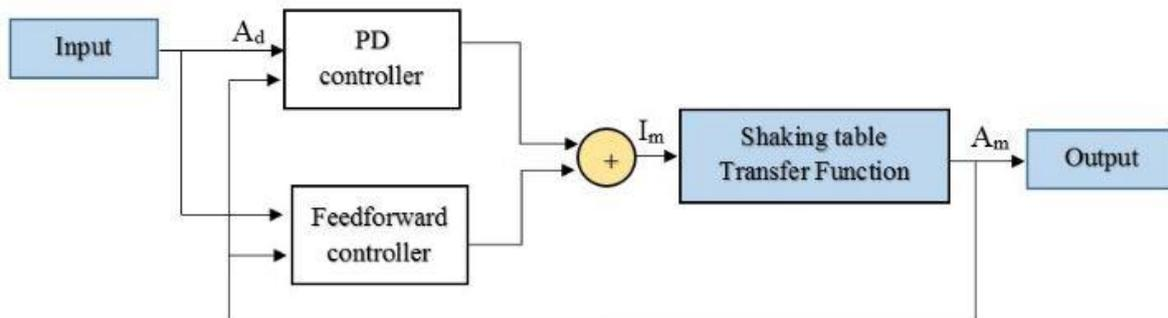
Fig. 2 – Simplified diagram of the shaking table and the original PDFF controller
