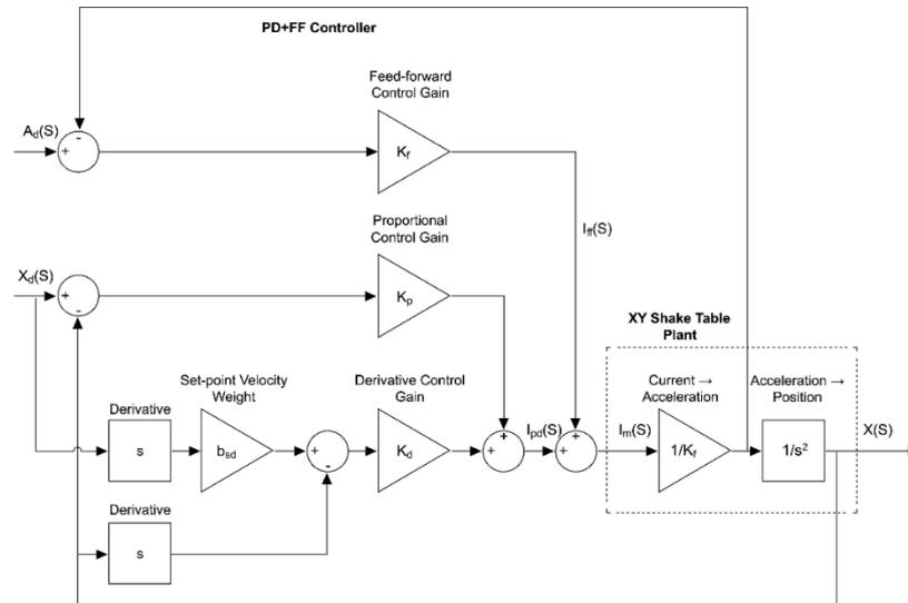
Fig. 3 – Schematic of the shaking table PDFF position controller
