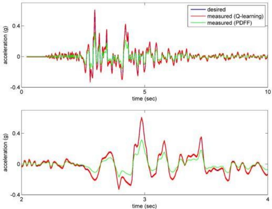
Fig. 6 – Numerical replication of Northridge earthquake record with the Q-learning and PDFF controller
