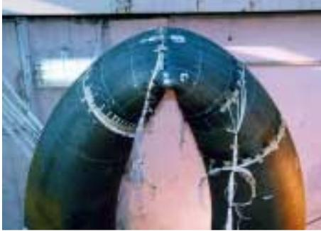
**Photo 1 Closing mode bending**
