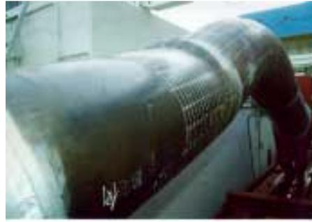
**Photo 2 Opening Mode Bending**
