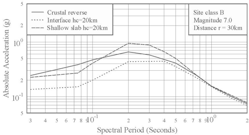
Figure 4. Comparison of reverse crustal, interface, and shallow slab spectra.
