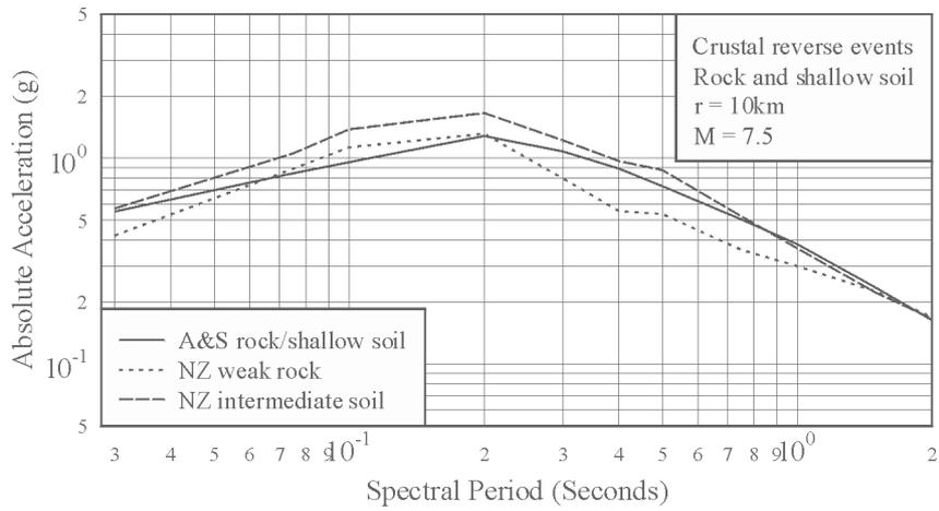
Figure 3. Near-source spectra at 10km for weak rock and shallow soil.
