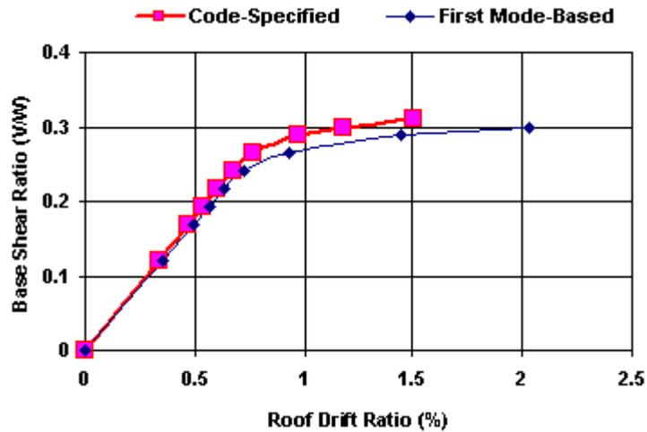
Figure 3: Base shear ratio vs. roof drift ratio
