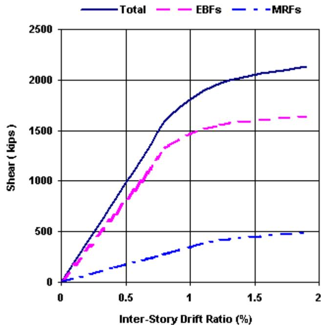
Figure 4: Story shear vs. inter-story drift ratio
