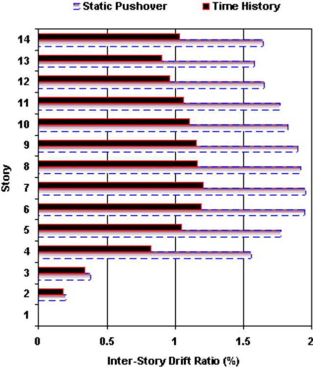
Figure 5: Envelopes of inter-story drift ratio
