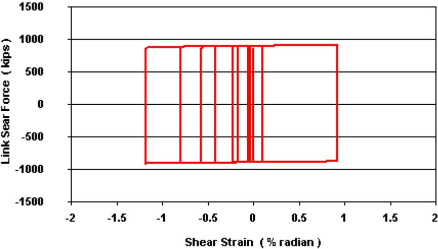
Figure 6: Shear force vs. shear strain in typical EBFs link
