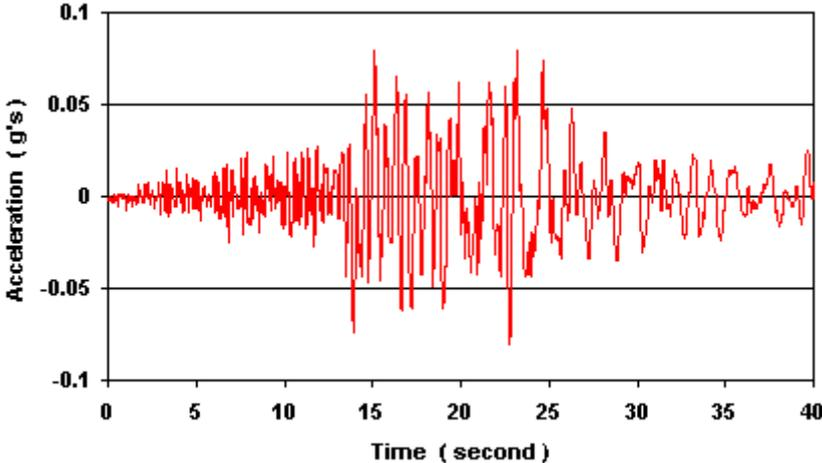
Figure 2: Recorded ground acceleration in Taipei Basin (CKS4012)
