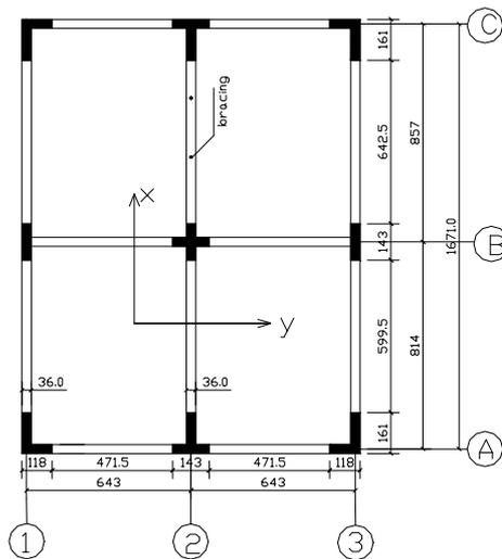
**Figure 1 The plan drawing**
