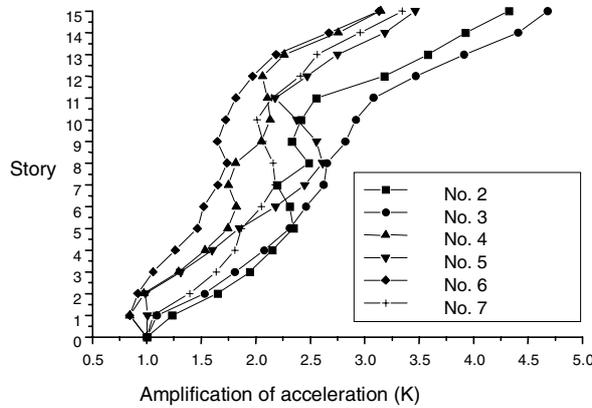
**Figure 6 Envelop diagram of K of the model**
